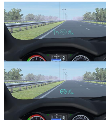
Figure 2. HUD warnings at work zone. Top: regular. Bottom: speeding.
