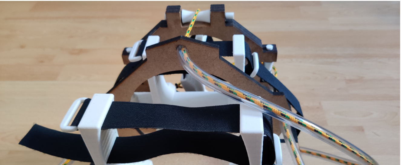
Figure 7.1.2. Top Bowden tube is in the way of the forearm fixation (when it is moved forward).
