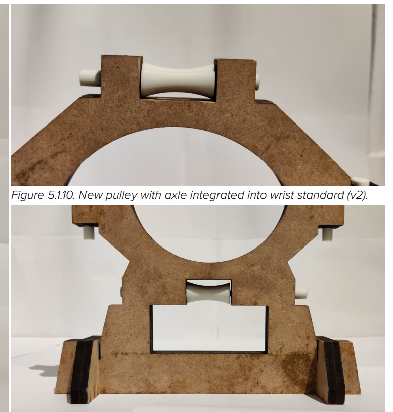
Figure 5.1.11. Wider wrist standard with supports more to the sides.
