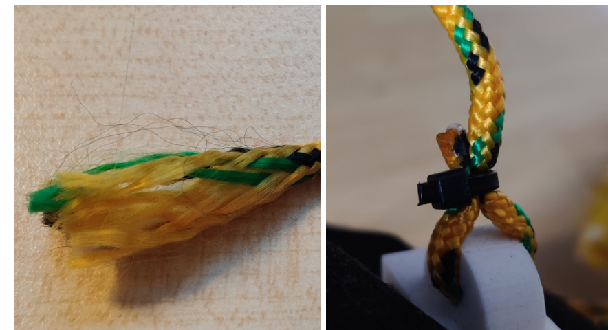
Figure 3.4.6. Disintegrated (left) and solidified end of the cable (right).
