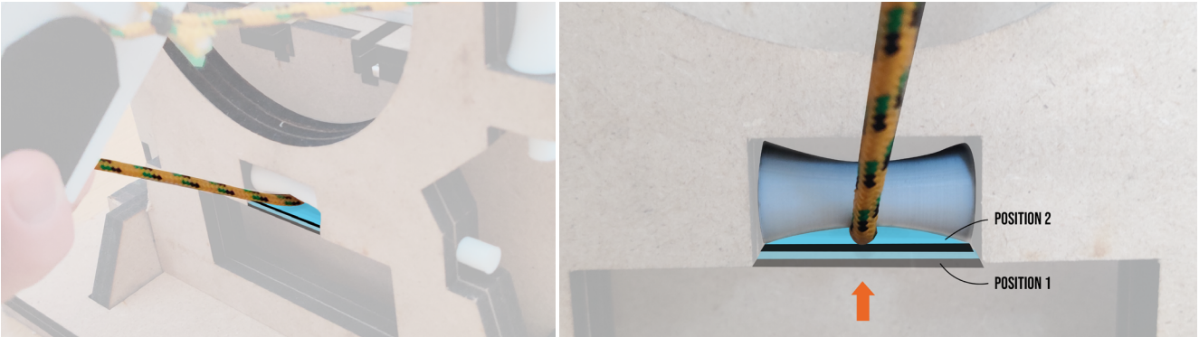
Figure 7.1.5. Roller underneath pulley and cable which can be pushed against cable to block it.
