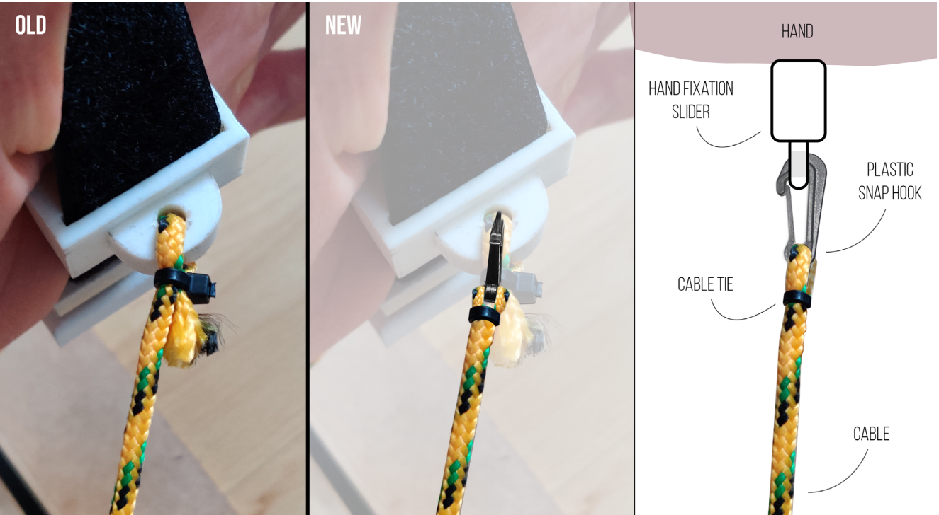
Figure 7.1.3. Old cable attachment with cable tie (left); new cable attachment with plastic snap hook (and cable tie) (right).
