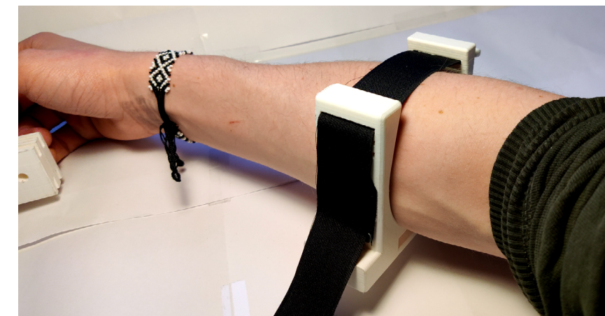
Figure 3.2.15. One strap velcro attachment loosened after applying pressure downwards.
