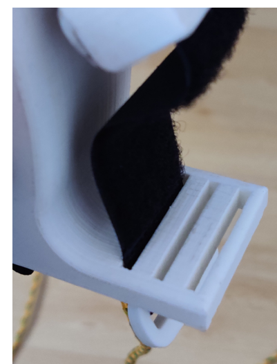
Figure 3.2.27. Different strap slots on hand fixation to account for variation in hand thickness.
