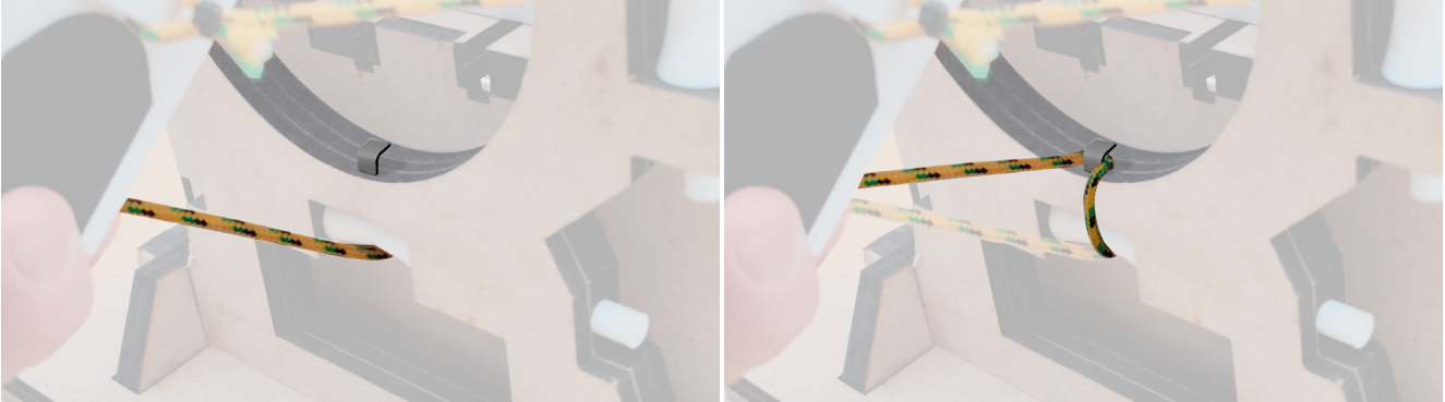
Figure 7.1.4. Small plastic hook used to secure the lower cable.
