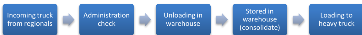
Figure 5-4: Export flow in Airmadidi dry port for general cargo and bag cargo Source: modified from (UNCTAD, 1991)
