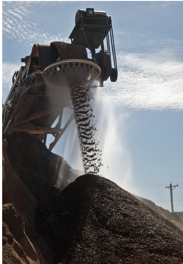
Figure 6.9: Water spray to suppress dust while discharging material [59]
