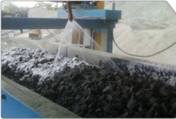
Figure 6.10: Foam sprayed on a conveyor to suppress dust [63]
