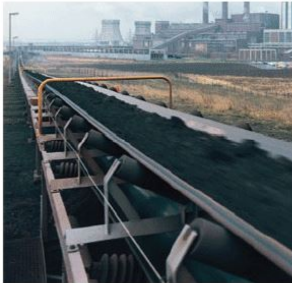
Figure 3.3: Through conveyor loaded with coal [24]
