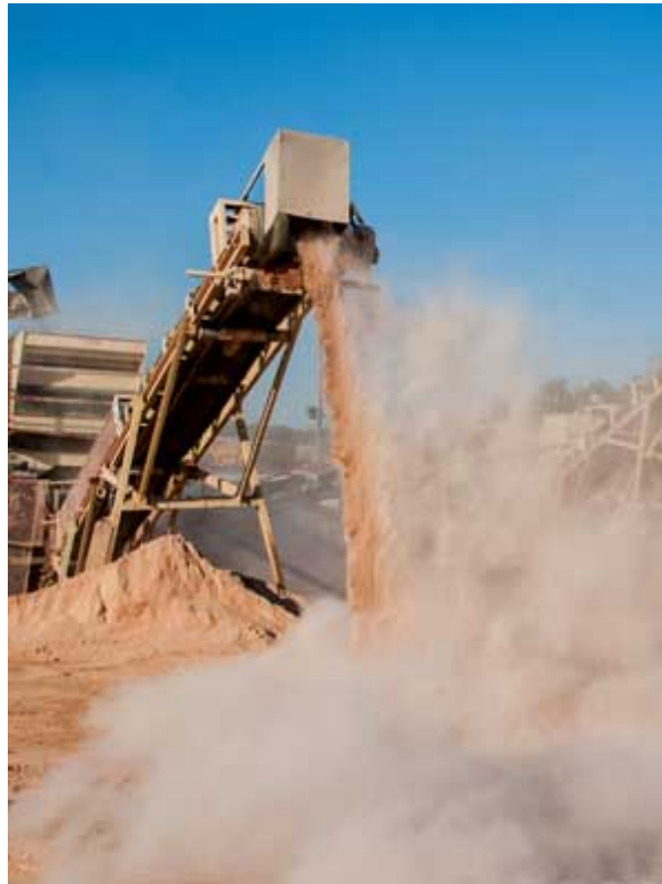
Figure 6.1: Dust generation during unloading [45]
