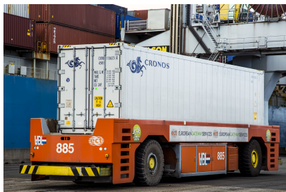
Figure 2-3: A loaded automated guided vehicle (AGV) transporting a two TEU container.
