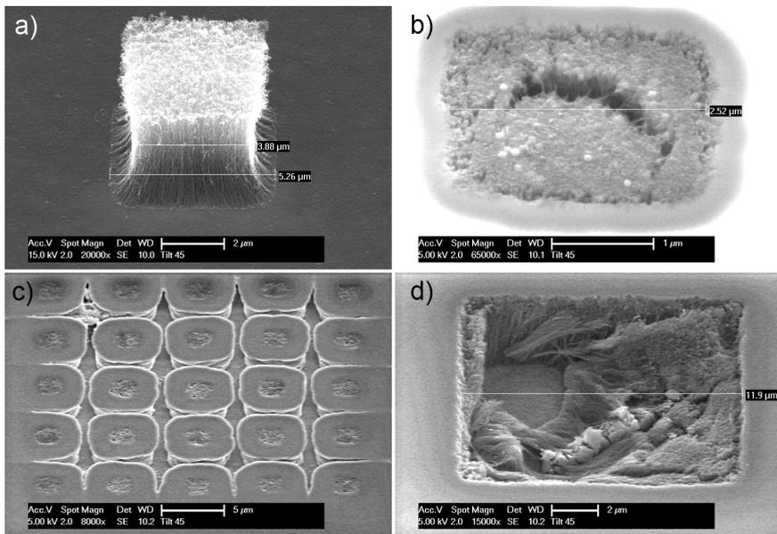
**Figure 4.15:** SEM images of: a) liquid densified bundle, b) densified bundle after CMP, c) array of bundles after CMP, d) large bundle after CMP displaying tube removal. Scale bars are: 2, 1, 5, and 2  $\mu\text{m}$ , respectively.
