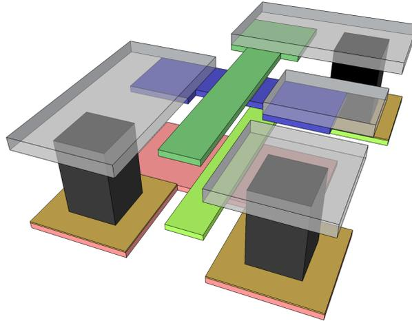
(a) Red: p-type Si, blue: n-type Si, green: gates, brown: Ti/TiN stack, black: CNT vias, grey: Al (1% Si). All layers thickness's and dimensions are to scale.
