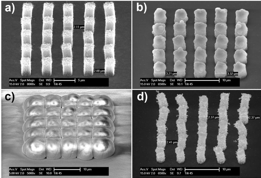
**Figure 4.13:** SEM images of: a) free-standing bundles grown on TiN (scale:  $5 \mu\text{m}$ ), b) bundles covered by  $1 \mu\text{m}$  TEOS (scale:  $10 \mu\text{m}$ ), c) bundles covered by  $5 \mu\text{m}$   $\text{SiO}_2$  (scale:  $10 \mu\text{m}$ ), d) bundles covered by  $200 \text{ nm}$   $\text{Si}_3\text{N}_4$  (scale:  $10 \mu\text{m}$ ).
