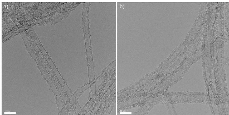
**Figure 4.9:** TEM images taken from samples grown at different conditions: a) 0.8 nm Fe, 50 mbar with 1000/50 sccm  $H_2/C_2H_2$  showing DWCNT with a diameter of 5 nm; b) 1.1 nm Fe, 80 mbar with 320/40 sccm  $H_2/C_2H_2$  showing MWCNT with a diameter of 8 nm. Scale bars are 10 nm.
