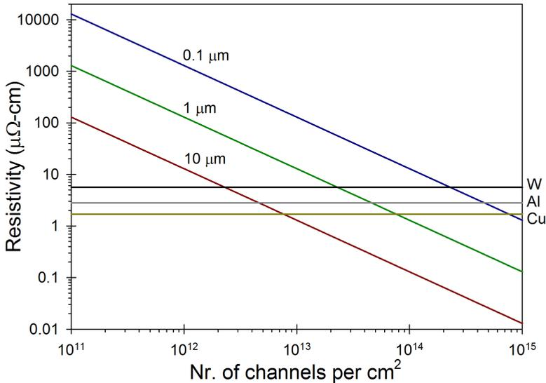
**Figure 2.7:** Minimum resistivity against nr. of channels for bundles with a different length. The MFP is assumed to be as long, or longer than, the bundle length.
