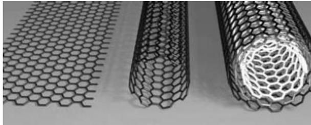
**Figure 1.3:** Schematic representation of (from left to right): graphene, SWCNT, and MWCNT.
