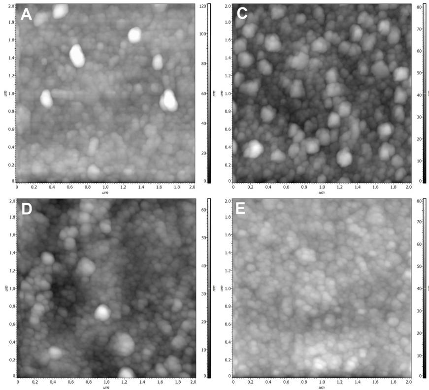
**Figure 4.18:** AFM images taken from samples A, C, D and E displaying the catalyst nanoparticles after activation. Area 2 by 2  $\mu\text{m}$ , height map in nm.
