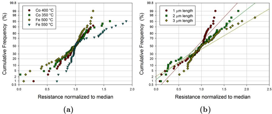
**Figure 5.3:** Cumulative frequency plots of: a) CNT vias grown at different temperatures, b) CNT via resistances of different length grown using Fe at 500 °C. Obtained from vias of 1.5  $\mu\text{m}$  width, all values are normalized to the median.
