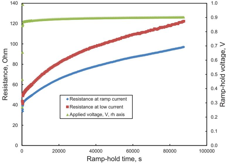
**Figure 5.16:** Complete 24 hours voltage hold test performed on 3  $\mu\text{m}$  wide via.
