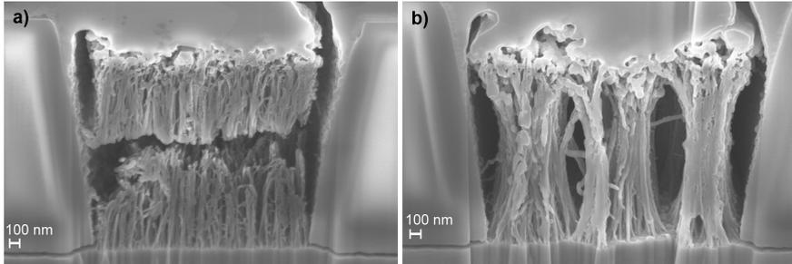
**Figure 5.14:** Post-mortem FIB cross-sections of  $2 \mu\text{m}$  vias: a) best performing via, b) typical early failure via.
