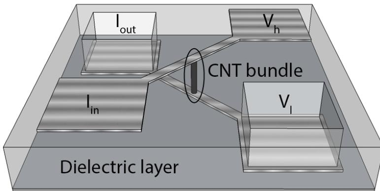
**Figure 4.10:** Sketch of a four-point probe measurements structure used to electrically characterize a CNT bundle.
