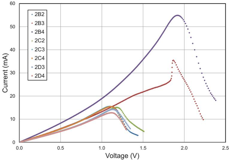
**Figure 5.12:** Ramp to failure tests on vias with a width of  $2 \mu\text{m}$ .
