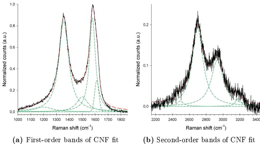
**Figure 3.7:** Fitted Raman spectra of CNF grown on 6 nm Ni at  $650\text{ }^\circ\text{C}$ . Original spectrum: solid line; fitting peaks: short dashed line (green); total fitting curve: long dashed line (red)
