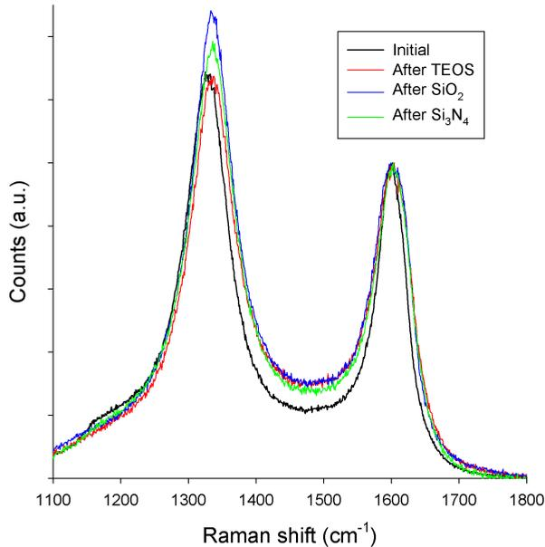
**Figure 4.14:** Raman spectra of CNT before and after covering with PECVD dielectrics. The intensity is normalized to the G-band.
