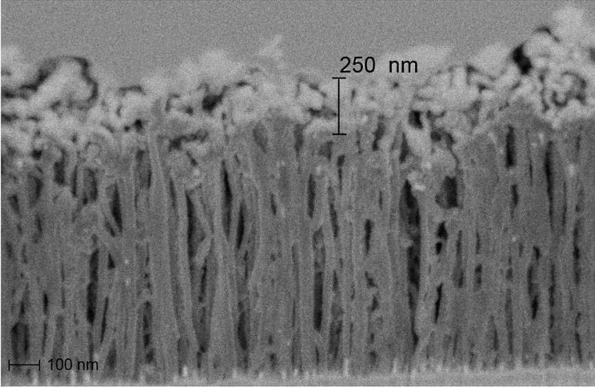
**Figure 5.5:** Close up of the CNT tips as imaged by the back-scatter electron detector in the dual-beam FIB/SEM, displaying a clear contrast between Ti and CNT.
