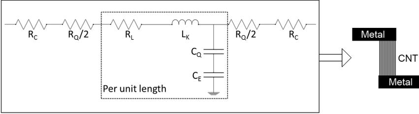
Figure 2.3: Equivalent circuit of a CNT bundle
