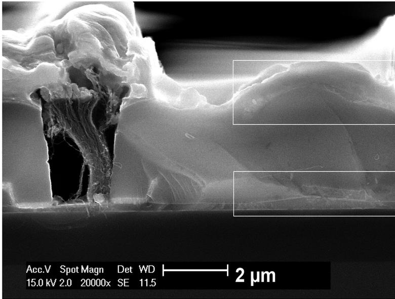
**Figure 7.5:** SEM image of a cross-section prepared using wafer cleaving. The square boxes indicate the position of the two SG-TFT.
