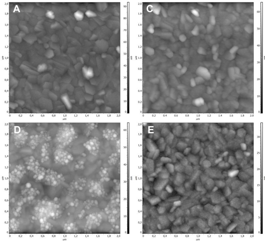
**Figure 4.17:** AFM images taken from samples A, C, D and E displaying the effect of the surface treatments on the TiN surface. Area 2 by 2  $\mu\text{m}$ , height map in nm.
