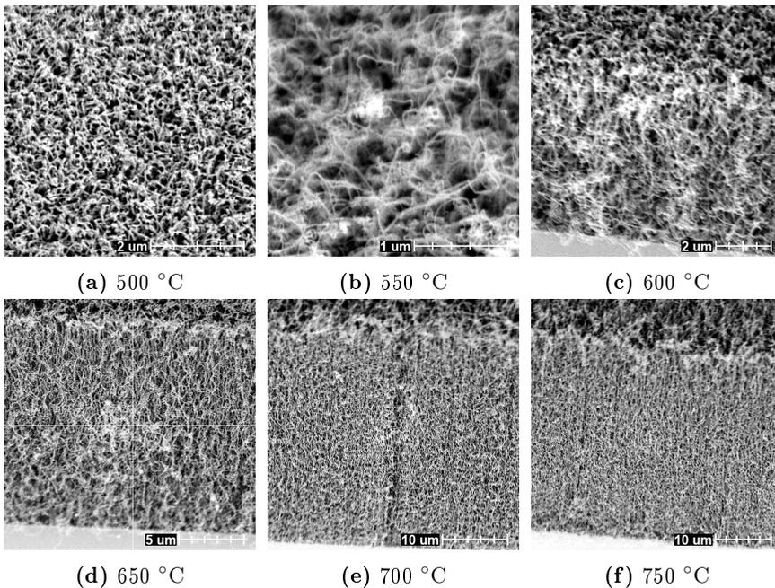
**Figure 3.1:** SEM images of MWCNT grown using 3 nm Fe at different temperatures
