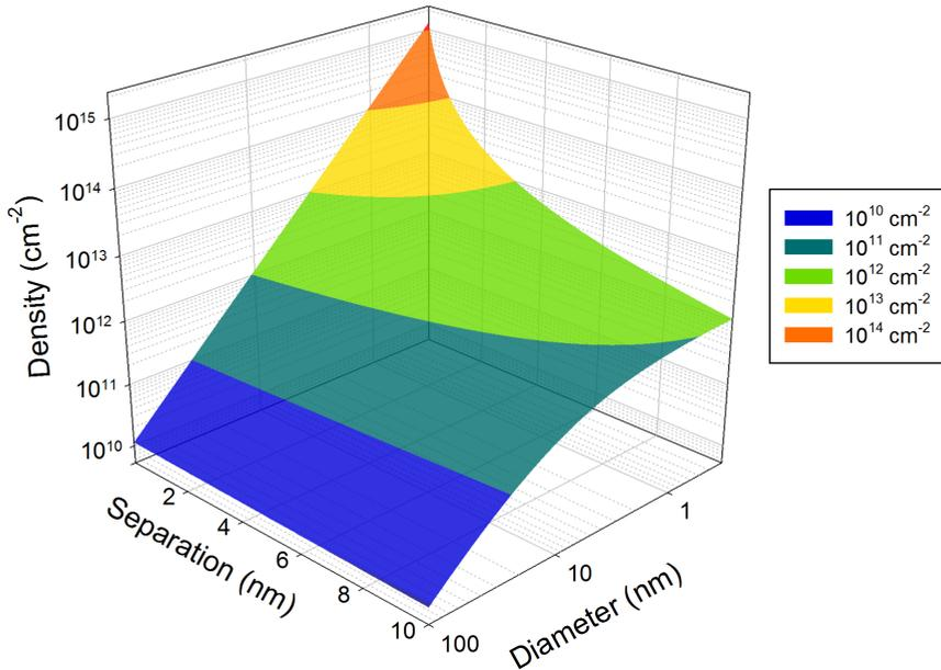
**Figure 2.5:** CNT density as predicted by the model against diameter and separation
