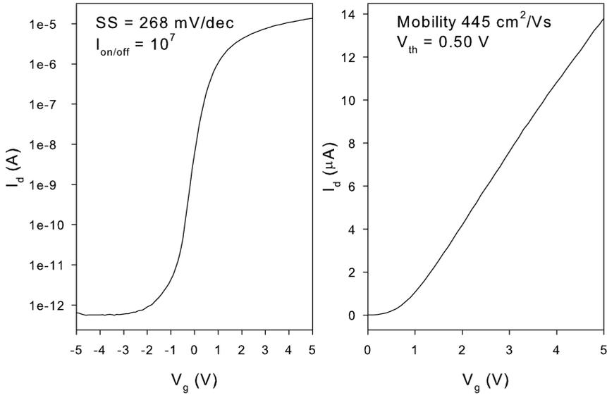
**Figure 7.7:**  $I_D$ - $V_G$  of a NMOSFET SG-TFT transistor with  $1 \mu\text{m}^2$  CNT vias.  $V_D = 0.1$  V.
