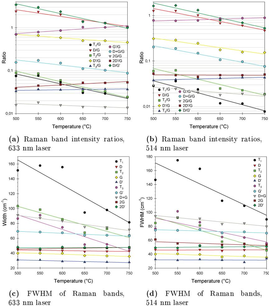
**Figure 3.8:** Results obtained from fitting the Raman spectra of MWCNT grown with 3 nm Fe at different temperatures
