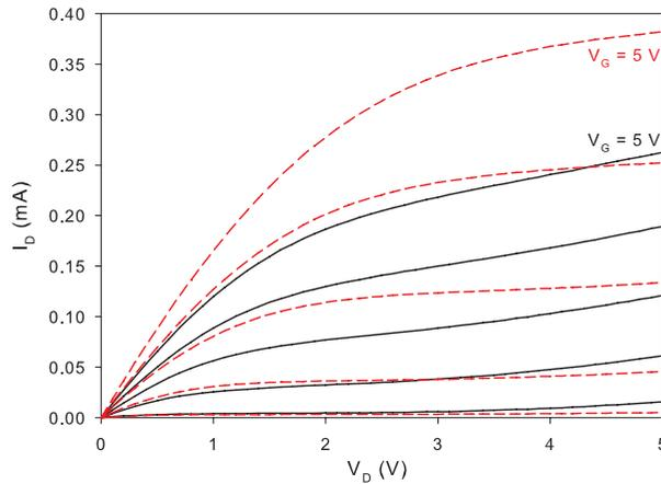
**Figure 7.9:**  $I_D$ - $V_D$  of a NMOS SG-TFT transistor with  $1 \mu\text{m}$  (solid line) and  $2 \mu\text{m}$  (dashed line) wide CNT vias.  $V_G$  ranges from 1 V to 5 V, in steps of 1 V.
