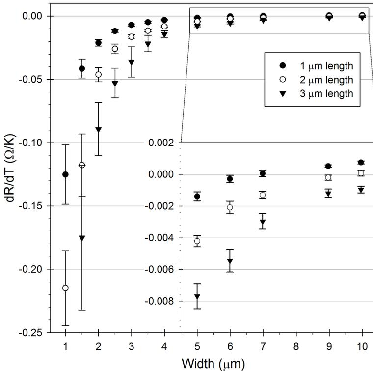
**Figure 5.9:** Thermal coefficient of resistance values for the measured temperature range, plotted for all via widths and lengths. The inset show a close-up of the vias ranging from 5-10  $\mu\text{m}$ .
