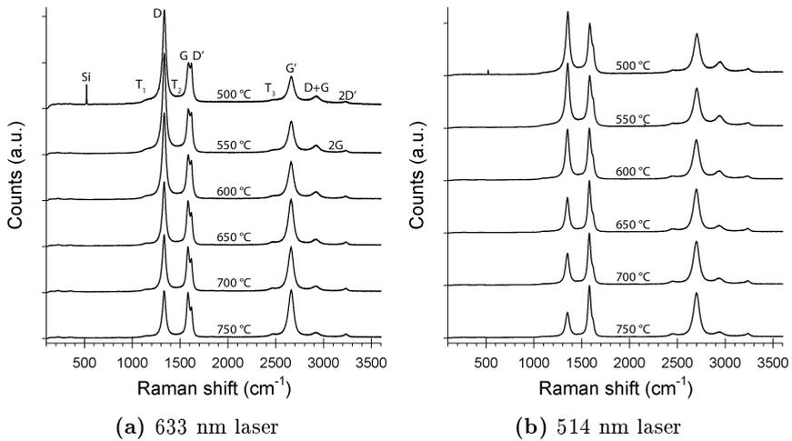
**Figure 3.4:** Raman spectra of MWCNT grown with 3 nm Fe, normalized to the G band intensity
