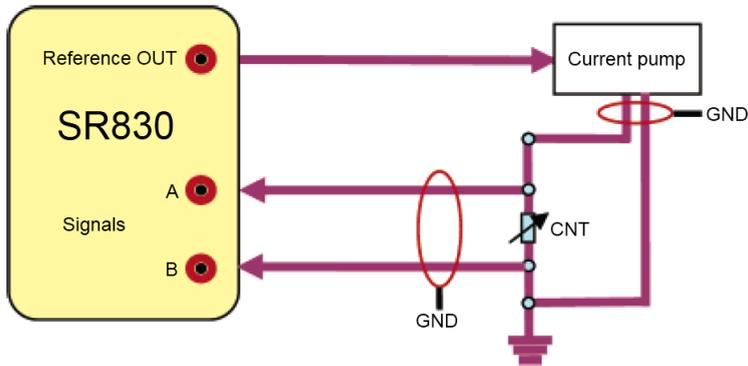
**Figure 6.1:** Schematic overview of the measurement setup.
