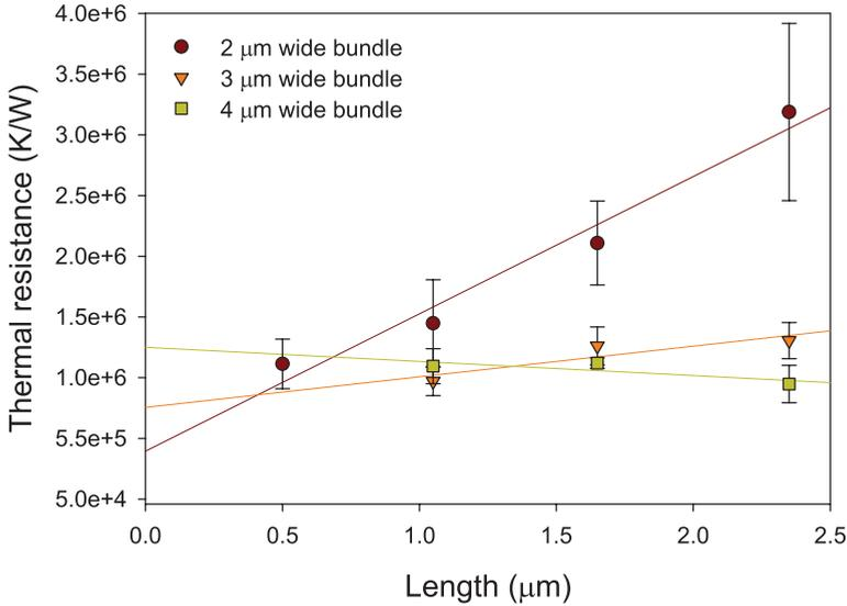
**Figure 6.5:** Average thermal resistance for each bundle length and width, plotted against the length of the bundle.
