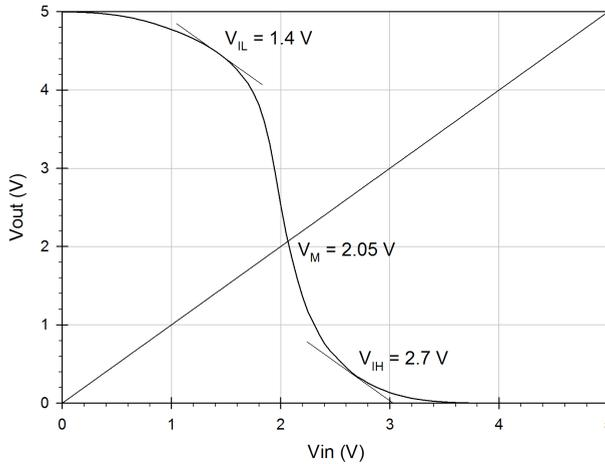
**Figure 7.10:**  $V_{in}$ - $V_{out}$  characteristics of a PMOSFET bottom 3D inverter with  $1 \mu\text{m}$  wide vias.
