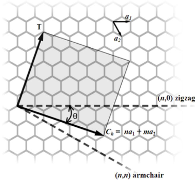
**Figure 2.1:** Definition of the chiral vector  $C_h$  and its indexes  $(n, m)$ .  $T$  denotes the tube axis, and  $a_1$  and  $a_2$  are the vectors of the graphene unit cell in real space.
