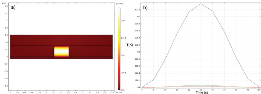
**Figure 6.2:** (Color online) Finite element simulation of via cross-section: a) temperature distribution at peak of sinusoid current, b) temperature at peak of sinusoid current at different locations in cross-section: centre of bundle (blue line), bottom electrode (green line), and top electrode (red line).
