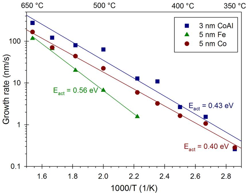
**Figure 4.4:** Arrhenius plot of the growth rate (in nm/s) against the inverse temperature for the different catalyst used in this work.
