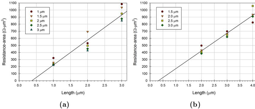
**Figure 5.6:** Resistance-area of smallest size CNT vias versus length, fabricated at 500 and 550 °C using Fe as catalyst
