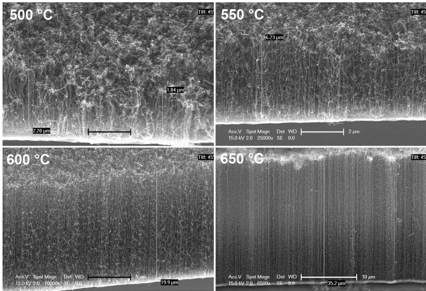
**Figure 4.1:** CNT grown using 5 nm Fe at different temperatures: 500 °C, 550 °C, 600 °C, and 650 °C. Growth time is 5 min for each sample. Scale bars are 1, 2, 5, and 10  $\mu\text{m}$ , respectively.
