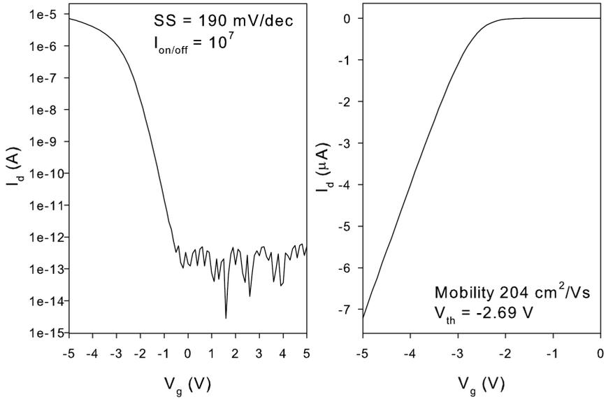
**Figure 7.8:**  $I_D$ - $V_G$  of a PMOSFET SG-TFT transistor with  $1 \mu\text{m}^2$  CNT vias.  $V_D = -0.1$  V.
