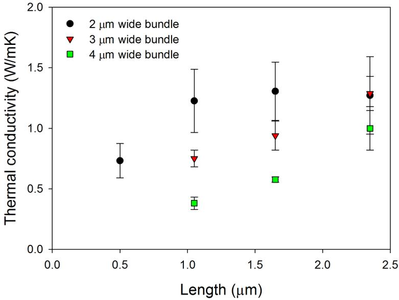
**Figure 6.6:** Average calculated thermal conductivity for each bundle length and width, plotted against the length of the bundle.
