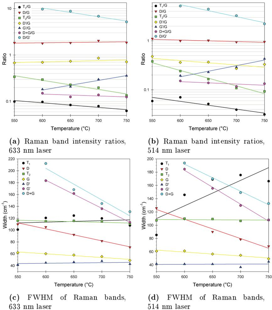
**Figure 3.9:** Results obtained from fitting the Raman spectra of CNF grown with 6 nm Ni at different temperatures
