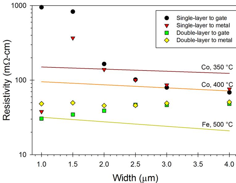
**Figure 7.6:** Calculated resistivities obtained from CNT vias to the bottom gate and metal levels from single and double layer processes, compared to result obtained in chapter 5.
