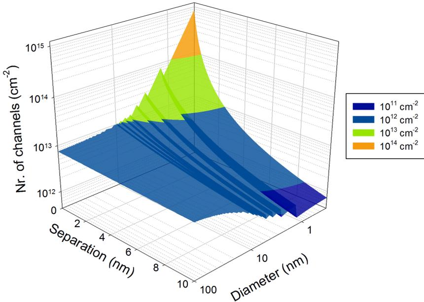
**Figure 2.6:** Calculated number of conductive channels of a CNT bundle as function of diameter and separation.
