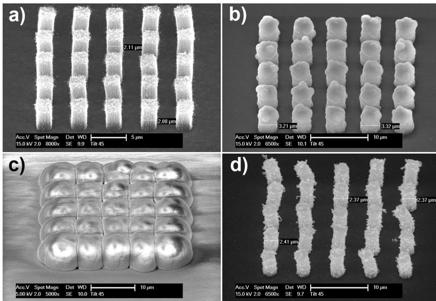
**Figure 4.13:** SEM images of: a) free-standing bundles grown on TiN (scale:  $5 \mu\text{m}$ ), b) bundles covered by  $1 \mu\text{m}$  TEOS (scale:  $10 \mu\text{m}$ ), c) bundles covered by  $5 \mu\text{m}$   $\text{SiO}_2$  (scale:  $10 \mu\text{m}$ ), d) bundles covered by  $200 \text{ nm}$   $\text{Si}_3\text{N}_4$  (scale:  $10 \mu\text{m}$ ).
