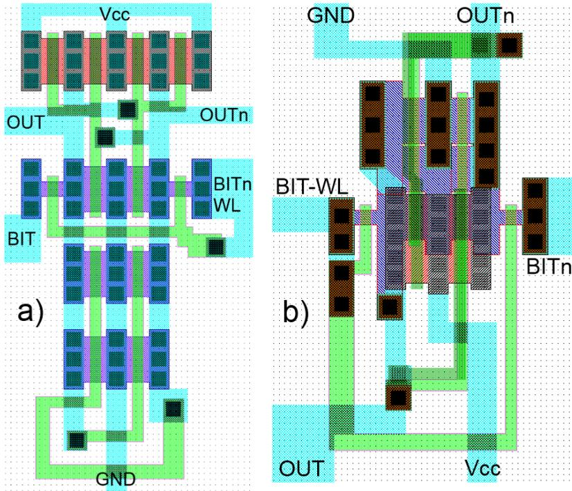
**Figure 7.11:** Mask lay-out of SRAM cells: a) single-layer; b) double-layer. Red: p-type Si, blue: n-type Si, green: gates, brown: Ti/TiN stack, black: CNT vias, grey: other contact openings, light blue: Al (1% Si), the grid spacing is  $1 \mu\text{m}$ .
