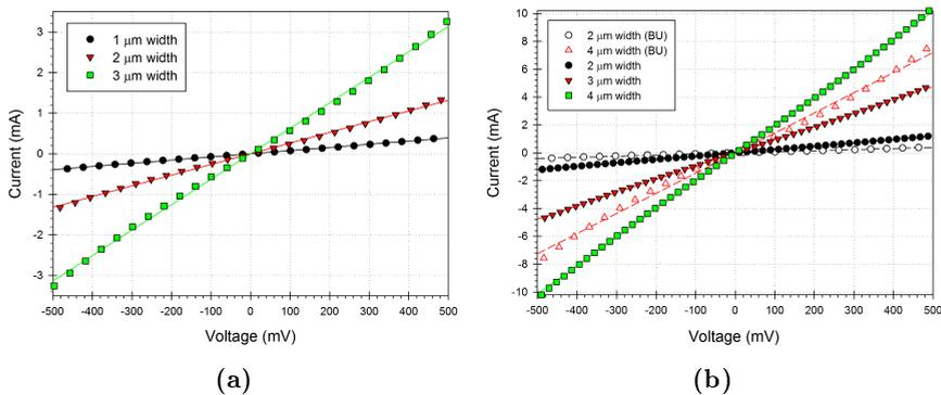
**Figure 5.1:** I-V characteristics obtained from: a) CNT grown at 350 °C, b) CNT grown at 500 °C using top-down and bottom-up (BU) approach.
