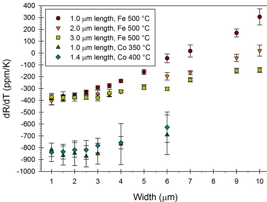
**Figure 5.10:** Thermal coefficient of resistance values for the measured temperature range in ppm/K, plotted for all via widths and lengths.
