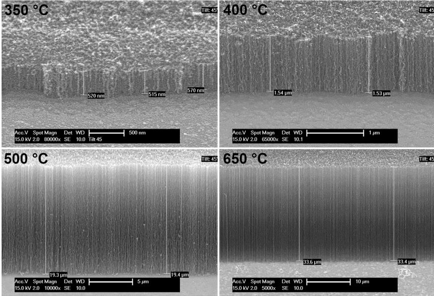
**Figure 4.2:** CNT grown using 3 nm Co-Al at different temperatures and growth times: 350 °C 30 min, 400 °C 10 min, 500 °C 5 min, and 650 °C 2 min. Scale bars are 0.5, 1, 5, and 10  $\mu\text{m}$ , respectively.
