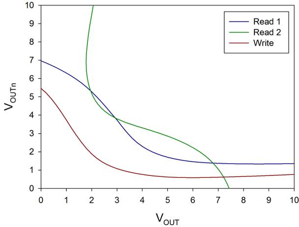
**Figure 7.12:**  $V_{OUT}$ - $V_{OUTn}$  characteristics of a 3D SG-TFT 6T-SRAM cell during read and write operations.
