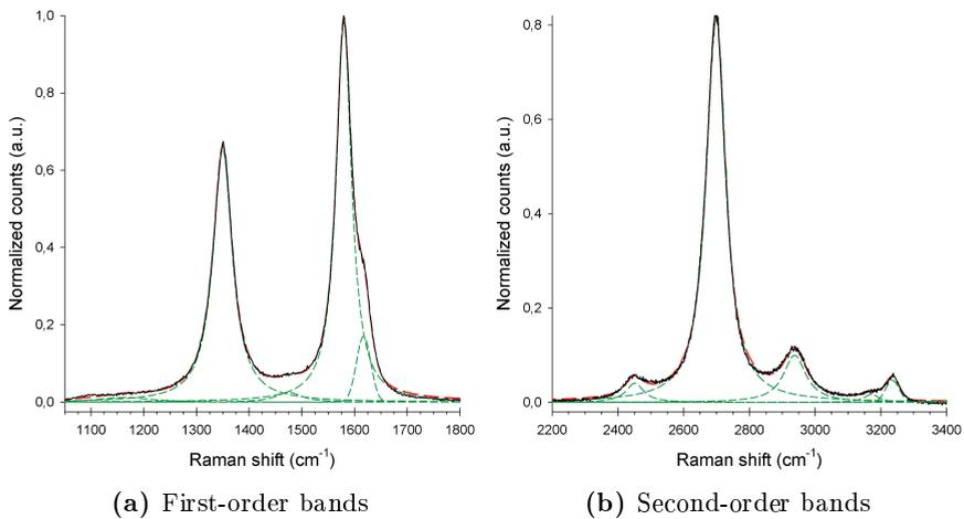
**Figure 3.6:** Fitted Raman spectra of CNT grown on 3 nm Fe at  $650 \text{ }^\circ\text{C}$ . Original spectrum: solid line; fitting peaks: short dashed line (green); total fitting curve: long dashed line (red)
