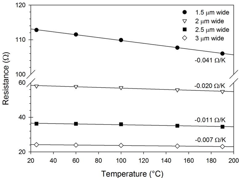
**Figure 5.8:** Resistance plotted against temperature for 1  $\mu\text{m}$  long CNT bundles of various widths. The solid line indicates a linear least squares fit.
