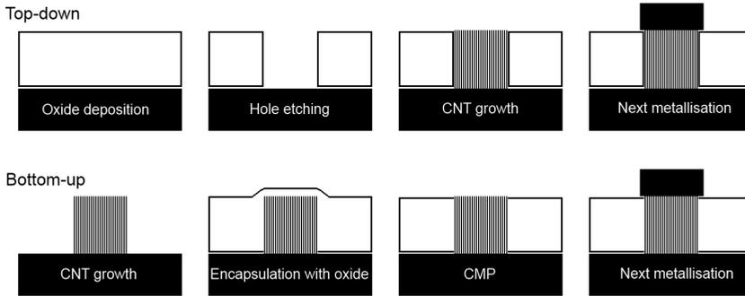
**Figure 4.12:** Schematic overview of top-down and bottom-up integration process
