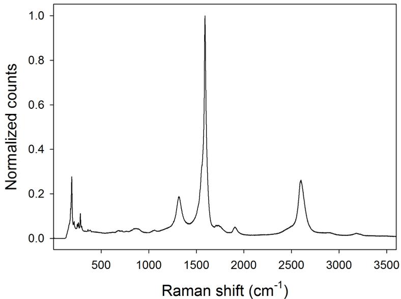
**Figure 4.8:** Raman spectrum of high quality CNT grown on ZrN with Fe as catalyst. The peaks around the low wavenumbers are the RBM of the CNT, of which the position depends on the diameter of the tube.
