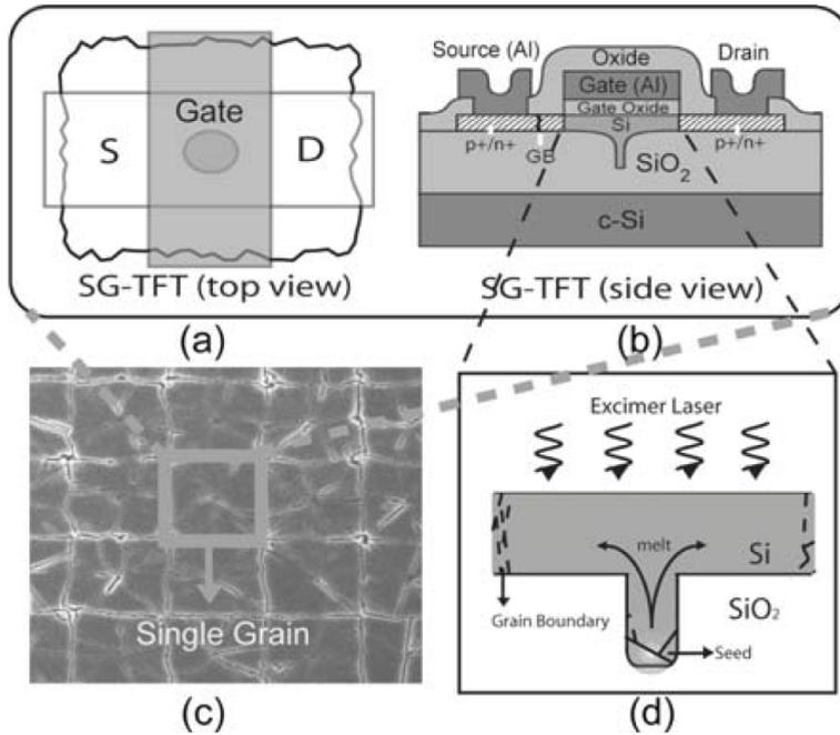
**Figure 7.1:** Overview of  $\mu$ -Czochralski SG-TFT process: a) SG-TFT top view, b) cross-section, c) SEM image of single-grains formed after laser crystallization, d) schematic of laser crystallization.
