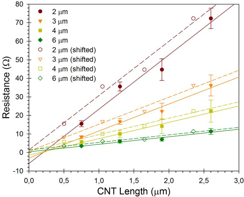
**Figure 5.4:** CNT bundle resistance vs. length for different bundle widths (2-6  $\mu\text{m}$ ). Closed symbols and solid line: measurement data corrected for approximate measured CNT length. Open symbols and dashed line: data shifted to take into account contact area.
