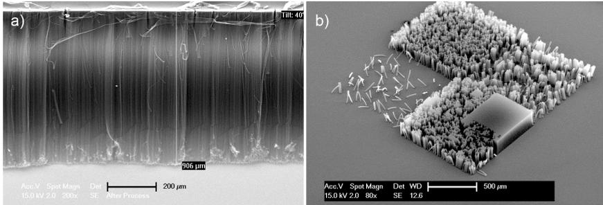
**Figure 4.7:** SEM images of optimized CNT growth on ZrN: a) optimum growth recipe with parameters as indicated in fig. 4.6, b) growth on area with random patterns with different fill factors. Scale bars are 200 and 500  $\mu\text{m}$ , respectively.
