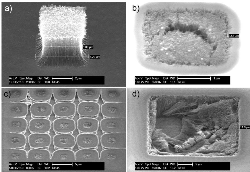
**Figure 4.15:** SEM images of: a) liquid densified bundle, b) densified bundle after CMP, c) array of bundles after CMP, d) large bundle after CMP displaying tube removal. Scale bars are: 2, 1, 5, and 2  $\mu\text{m}$ , respectively.
