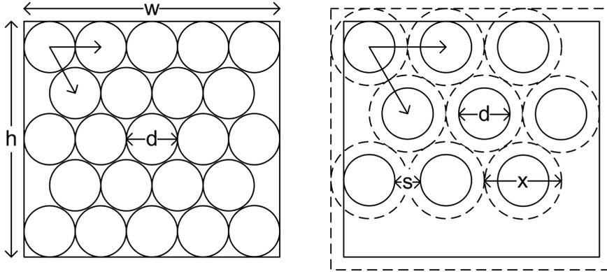
**Figure 2.4:** Model of ideal tight packed (left) and sparse packed (right) bundle
