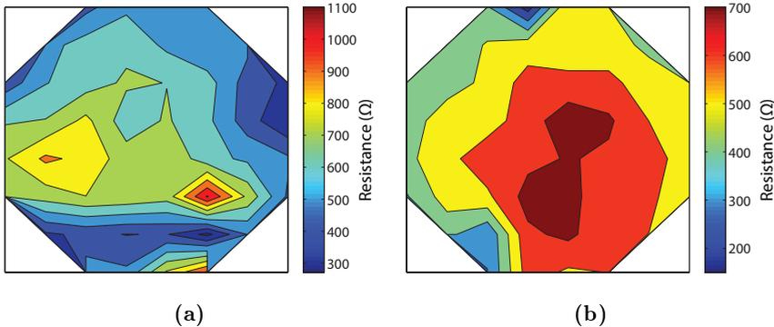
**Figure 5.2:** Resistance contour plot obtained from 1.5 μm wide CNT vias fabricated at: a) 350 °C, and b) 400 °C.
