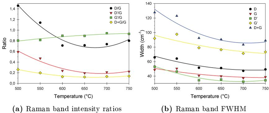
**Figure 3.10:** Results obtained from fitting the Raman spectra of MWCNT grown with 10 nm Fe at different temperatures using alternative growth recipe. Laser wavelength 514 nm.
