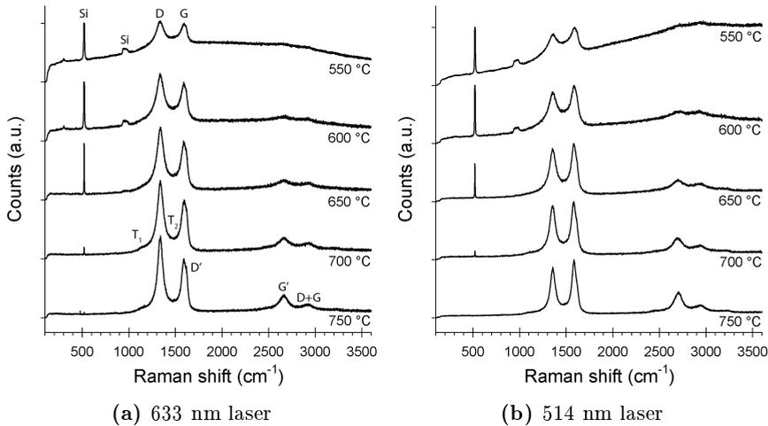
**Figure 3.5:** Raman spectra of CNF grown with 6 nm Ni, normalized to the G band intensity
