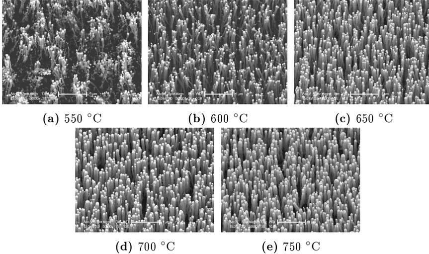
**Figure 3.3:** SEM images of CNF grown using 6 nm Ni at different temperatures, scale bar is 1  $\mu\text{m}$  for all images
