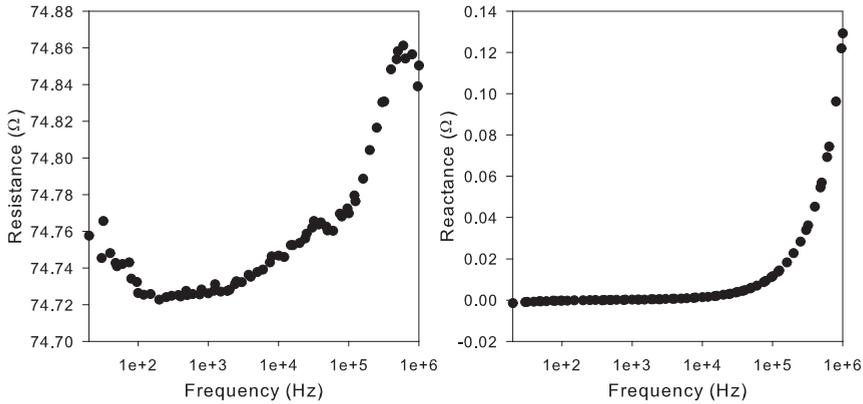
**Figure 6.3:** Impedance spectra of a typical  $2 \mu\text{m}$  wide via obtained using a LCR-meter.
