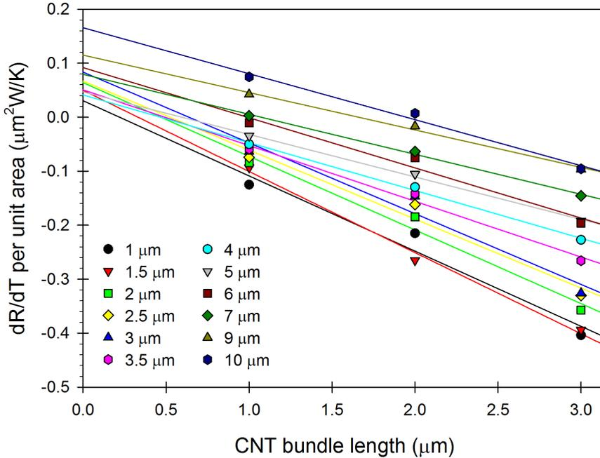
**Figure 5.11:** TCR normalized per unit area plotted against length. Each solid line represent a linear least squares fit.
