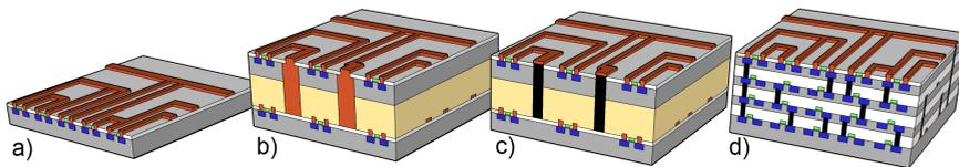
**Figure 1.2:** Overview of current and future interconnect technology: (a) traditional planar technology, all metal layers are routed on top of the transistors; (b) current 3D IC technology using Cu TSV to connect chip or wafer stacked layers of transistors; (c) 3D IC TSV technology with CNT TSV; (d) monolithic 3D IC with high aspect ratio CNT vias
