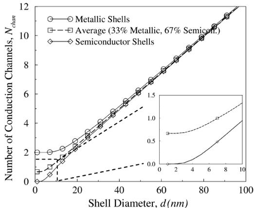
**Figure 2.2:** Number of conductive channels per wall vs. diameter ( $T = 300 \text{ K}$ ), from [49]
