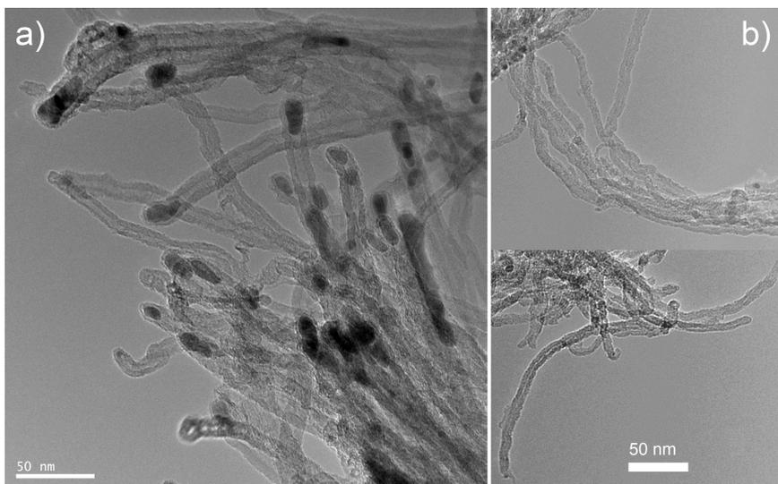
**Figure 4.3:** Typical TEM images taken from: a) 500 °C Fe grown samples, b) 350 °C Co grown samples.
