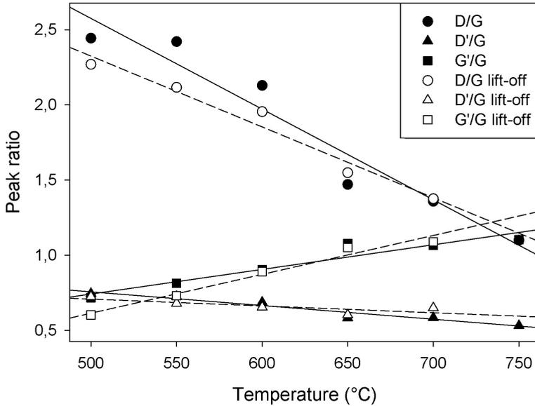
**Figure 4.11:** Raman band ratios comparison for CNT grown at different temperatures using Fe on TiN, patterned by lift-off, compared to non-patterned samples
