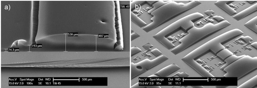
**Figure 4.5:** Growth issues with ZrN when the standard LPCVD recipe is used: a) edge of the wafer, where the Fe catalyst thickness gradually decreases due to local shielding displaying the sensitivity to catalyst thickness; b) loading effects occurring in patterned samples. Scale bars are 500  $\mu\text{m}$ .
