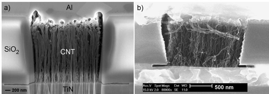
**Figure 4.19:** SEM cross-sections of CNT test vias: a) FIB prepared sample of 2.6 μm long via grown at 500 °C using Fe (54° tilt); b) mechanically cleaved sample of 1 μm long via grown at 350 °C using Co.
