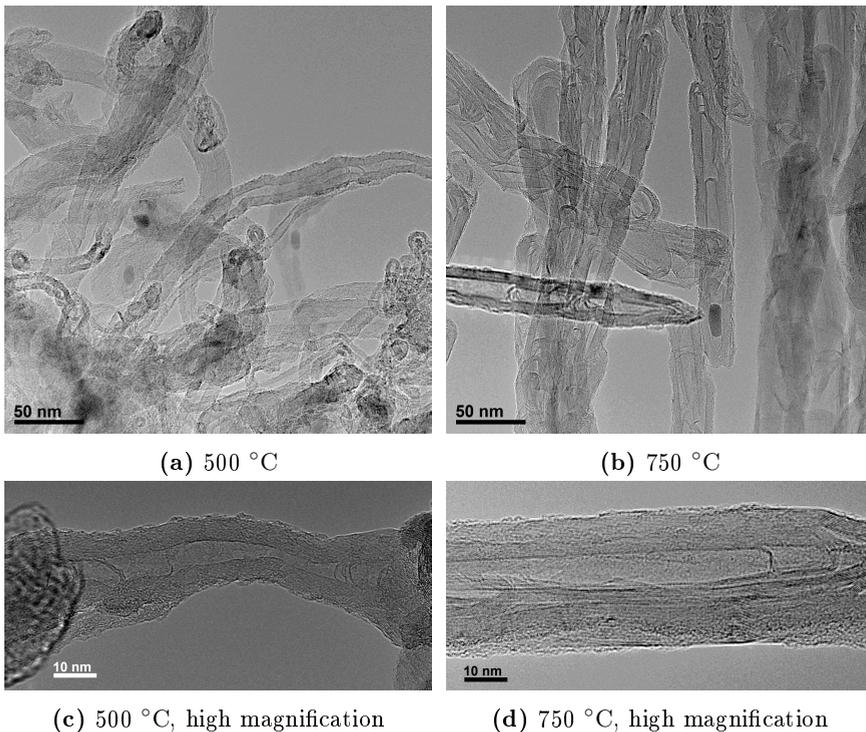
**Figure 3.2:** TEM images of MWCNT grown using 3 nm Fe at 500 and 750 °C
