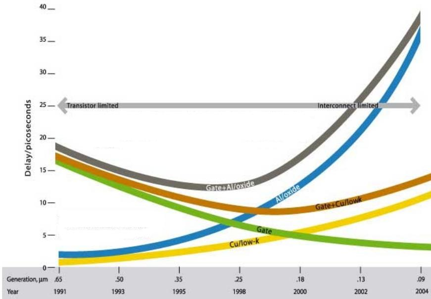
Figure 1.1: Gate and interconnect delay for different technology nodes, source [2]
