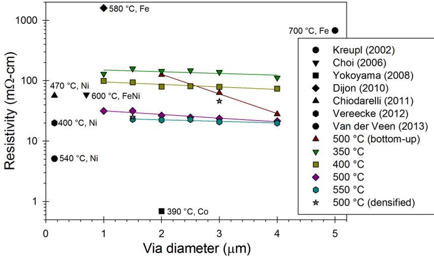
**Figure 5.7:** Resistivity from samples fabricated at different temperatures, compared with values obtained from literature.
