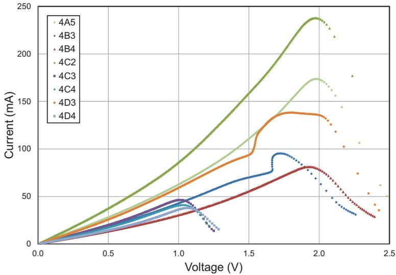
**Figure 5.13:** Ramp to failure tests on vias with a width of  $4 \mu\text{m}$ .
