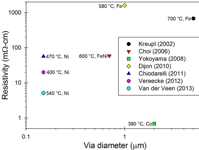
**Figure 1.4:** Overview of reported electrical performance of fully integrated CNT vias from literature.
