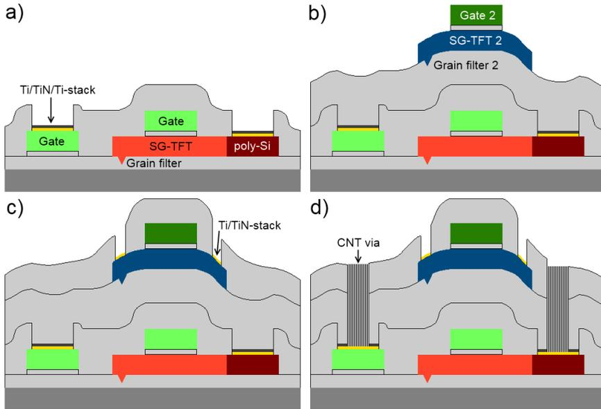
**Figure 7.3:** Cross-sectional view of final 3D SG-TFT process: a) after SG-TFT formation and deposition of Ti/TiN/Ti-stack; b) after fabrication of second-layer SG-TFT; c) after deposition of Ti/TiN oxidation barriers; d) after growth of CNT vias, before metallization. Layer thicknesses are not to scale.
