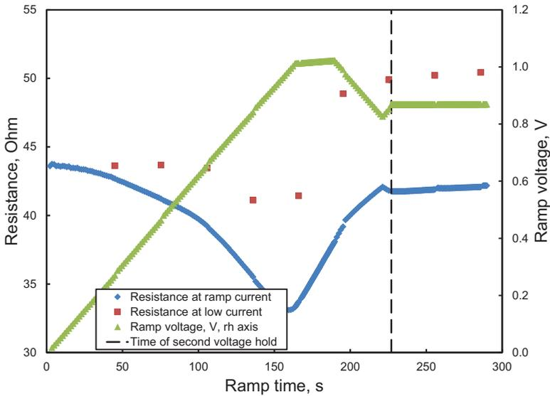
**Figure 5.15:** Start of voltage hold test performed on  $3\ \mu\text{m}$  wide via.
