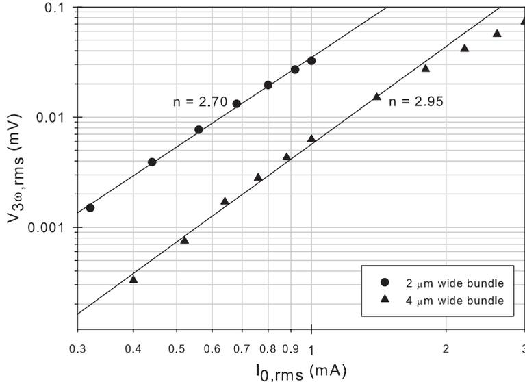
**Figure 6.4:** Measured third harmonic as function of the applied current.
