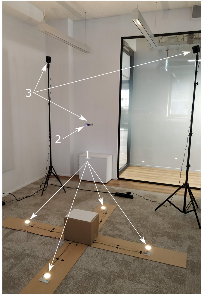
Figure 4.3: The overview of the system. The physical position of the testbed with 1) 4 transmitters; 2) UAV; and 3) the ground truth system. [8]
