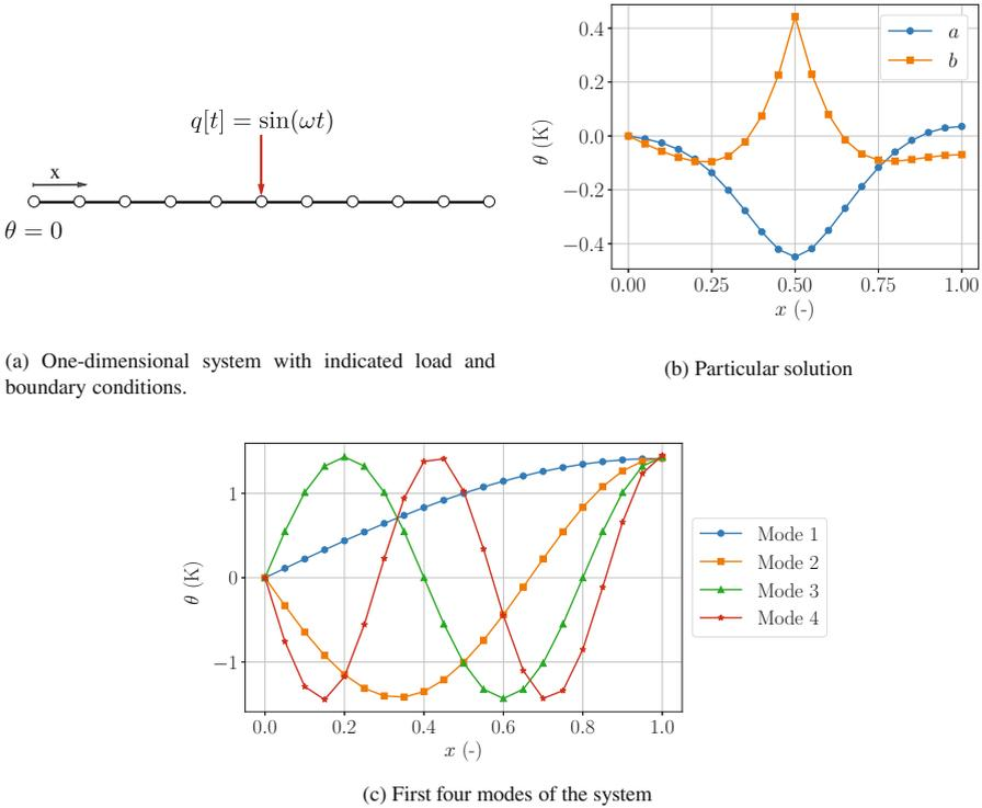
**Fig. 1.** Illustration of a one-dimensional bar with the applied boundary conditions (a), and the resulting temperature distributions corresponding to the particular solution (b). The first four thermal modes are visualized in (c).
