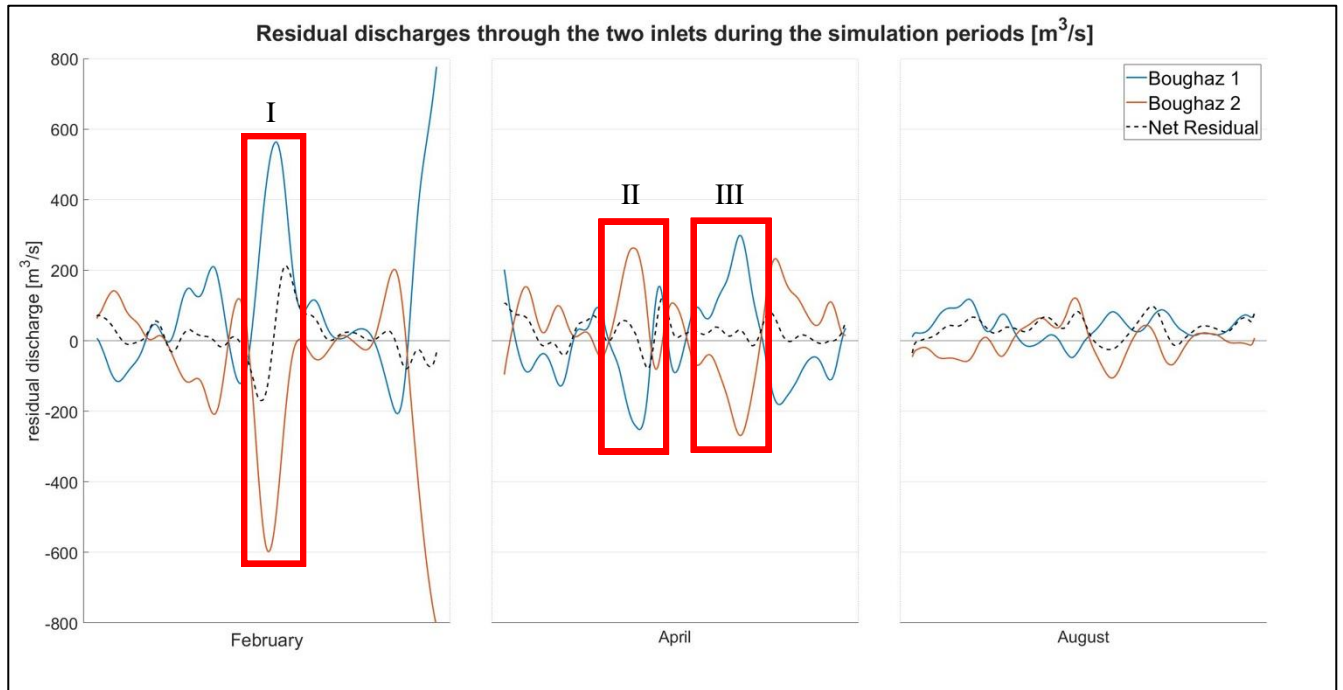
Figure 22: Residual discharges [ \text{m}^3/\text{s} ] through the two inlets during the simulations of the status quo. From left to right showing the inlet specific residuals (blue & orange) and net residuals (black) for the months of February, April, August
