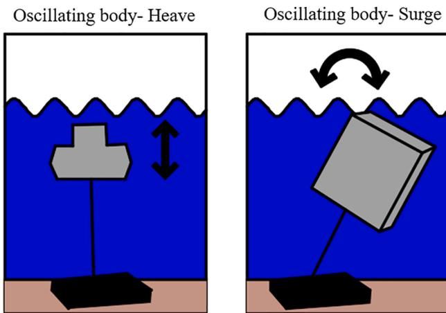
Fig. 9. Wave-activated bodies applicable to hybrid concepts.
