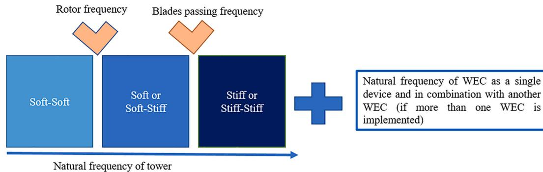
Fig. 4. Possible design windows for hybrid concepts base on the relative natural frequencies for wind turbine inspired by [77].
