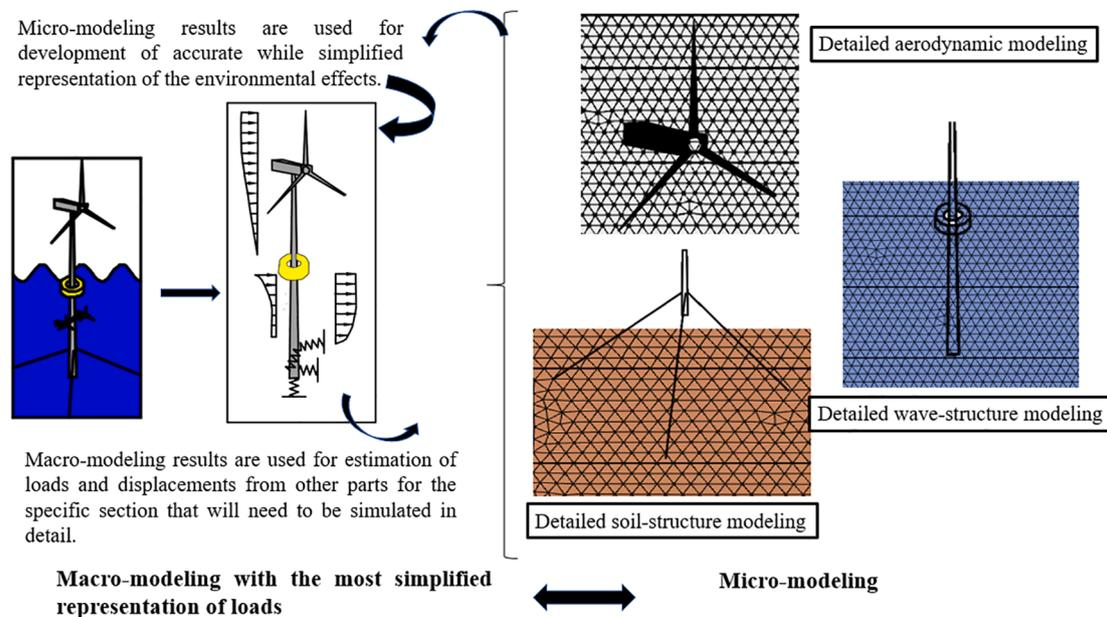
Fig. 5. Exemplary sketch of multi-level micro-and macro-modelling.
