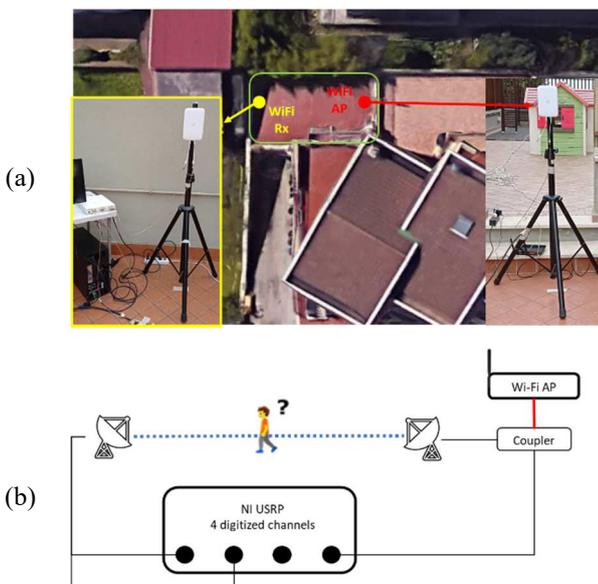
Figure 5. Experimental setup for the 2<sup>nd</sup> measurement campaign: (a) acquisition geometry, (b) sketch of the setup and components.
