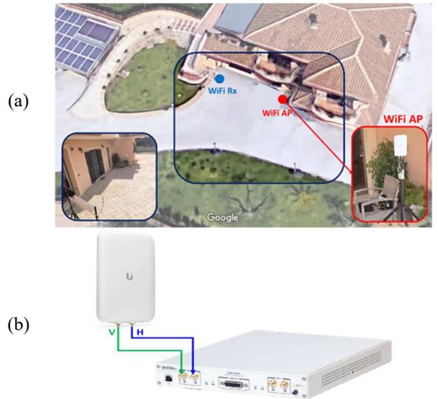
Figure 2. Experimental setup for the 1<sup>st</sup> measurement campaign: (a) acquisition geometry; (b) dual-polarimetric antenna and USRP used as receiver.
