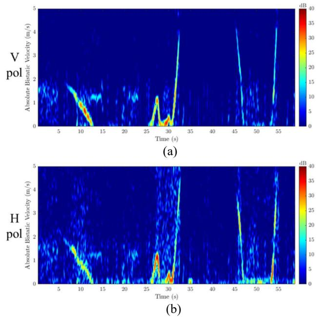
Figure 3. Output spectrograms obtained for the experimental test with the small drone, for the two pol channels, i.e., V (a) and H (b).
