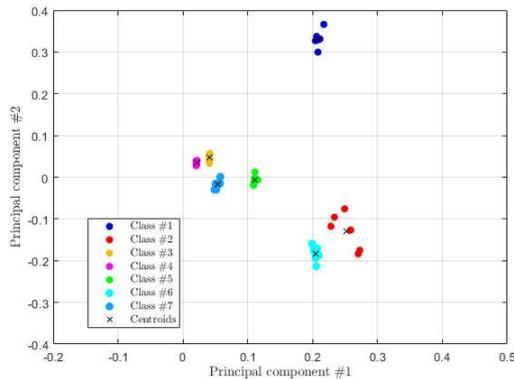
Figure 10. Output of the PCA with two features applied on the joint data from both polarimetric channels.
