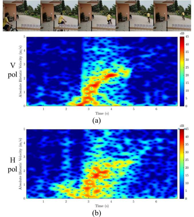
Figure 4 Test with bicycle: video frames of the exploited test (top) and output spectrograms obtained for the two pol channels, i.e., V (a) and H (b).
