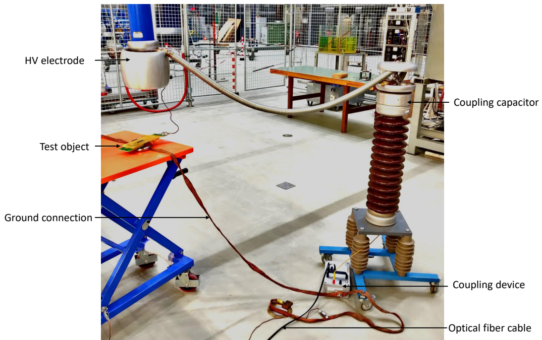
Figure 6.6: Straight-detection type partial discharge test setup
