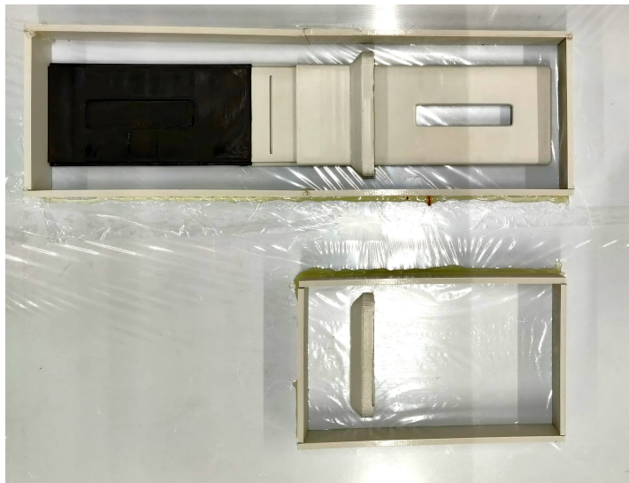
Figure 6.1: 3D model for silicon rubber casting
