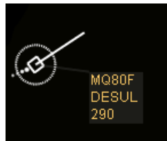
Figure 5: Aircraft label colour changes when aircraft received a command and is manoeuvring.
