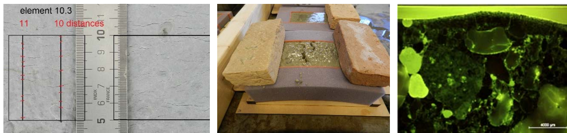
Figure 6: (left) Visual inspection; (right) mini-deformation tests and microscopic investigation
