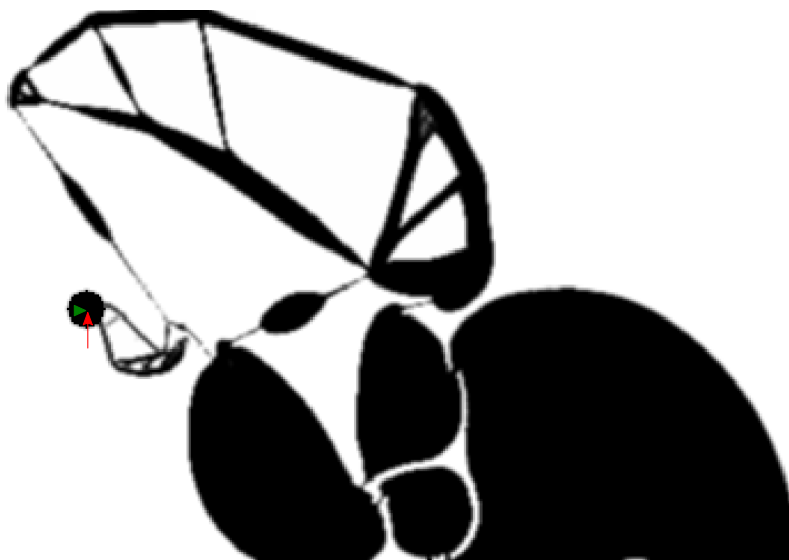
Figure A.3: Final result of CT Extreme 8 where the filter radius is incrementally decreased.
