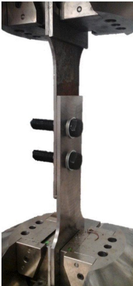
Fig. 5. Fatigue test on single shear bolted connection.
