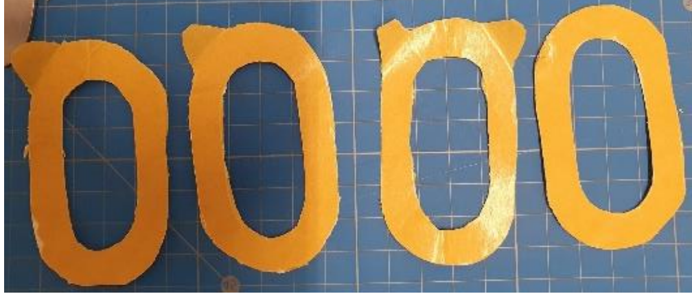
Figure 3.42: First, it was tried to pull the sheet using tabs. However, this only worked for perpendicular tensile forces, which were impossible to perform in practice
