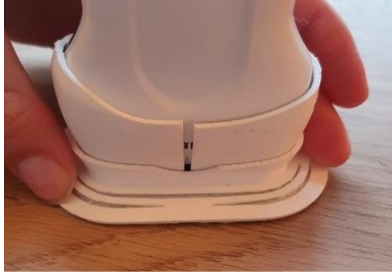
4. Figure 3.66: Push outer ring, with adhesive underneath, down to lock device
