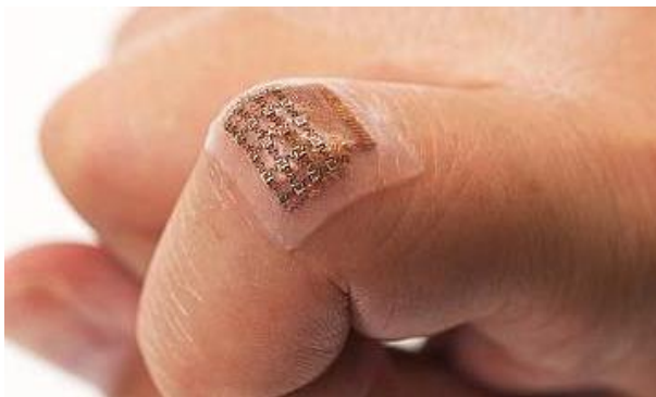
Figure 1.8: the wireless, flexible silicone patch for hemodynamic monitoring by the University of California. This is a non-working prototype, the patch still requires wires for power [30].
