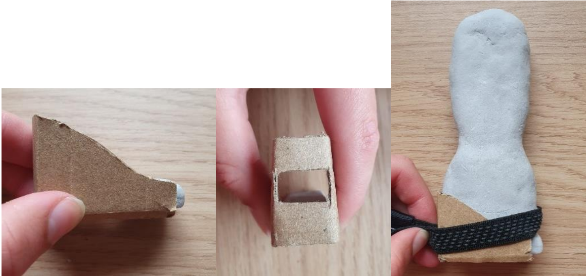
Figure 3.12a t/m d: recreating ideas from cardboard, clay and hairbands. The models showed there is no place for wires in this design. Therefore, a hole was made. However, these tests pointed out that a design containing elastic bands is not providing a secure fit.
