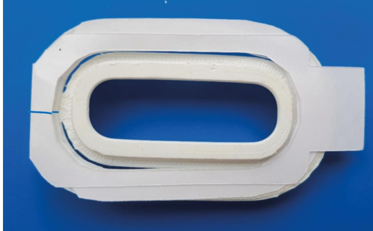
Figure 3.47: Plaster and protection sheet on gel pad holder. The double-struck part of the protection sheet attached to the plaster because of the cutouts in the other half of the protection sheet.
