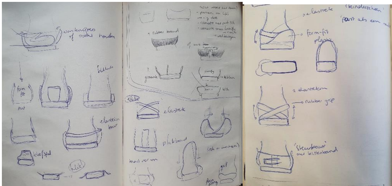
Figure 3.11: ideation drawings of how to connect the Lumify to the gel pad, and how to disconnect again. To allow for attachment and detachment, some kind of elastic force should be used. These drawing ideas were translated to cardboard mockups.
