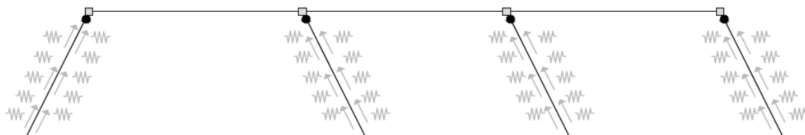
Figure 40: Schematization of raking piles
