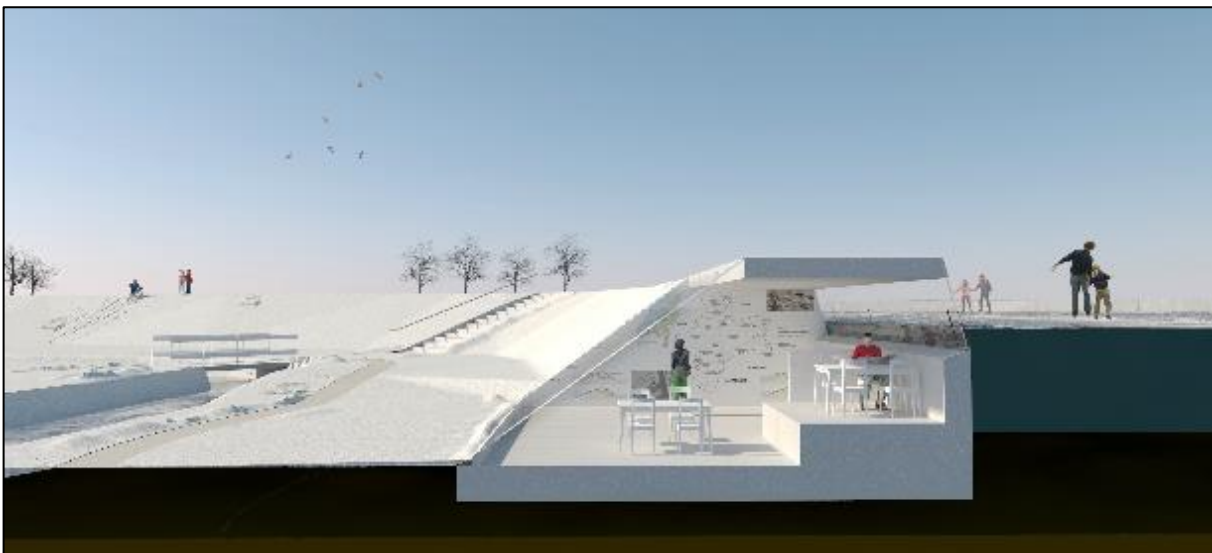
Figure 2: Cross-section of glass dike (De Architect, 2014)
