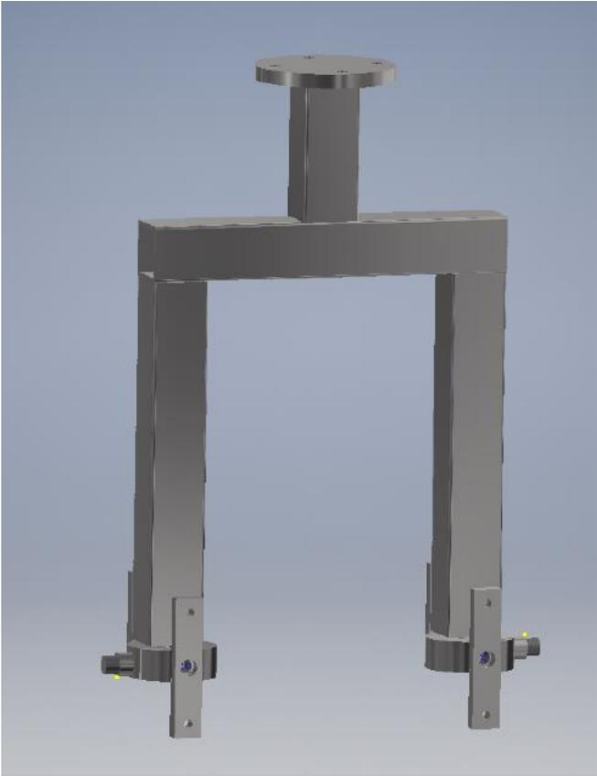
Figure 83: Chain holder (drawing by B.A. van den Bosch)
