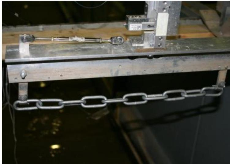
Figure 8: Test setup with long linked chain (Enerhaug, 2011)
