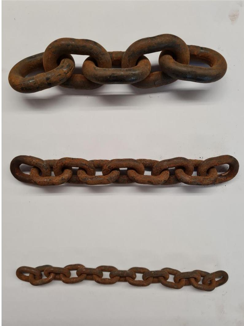
Figure 44: Three different chain link diameters, from top to bottom: 16 mm, 10 mm, 6 mm
