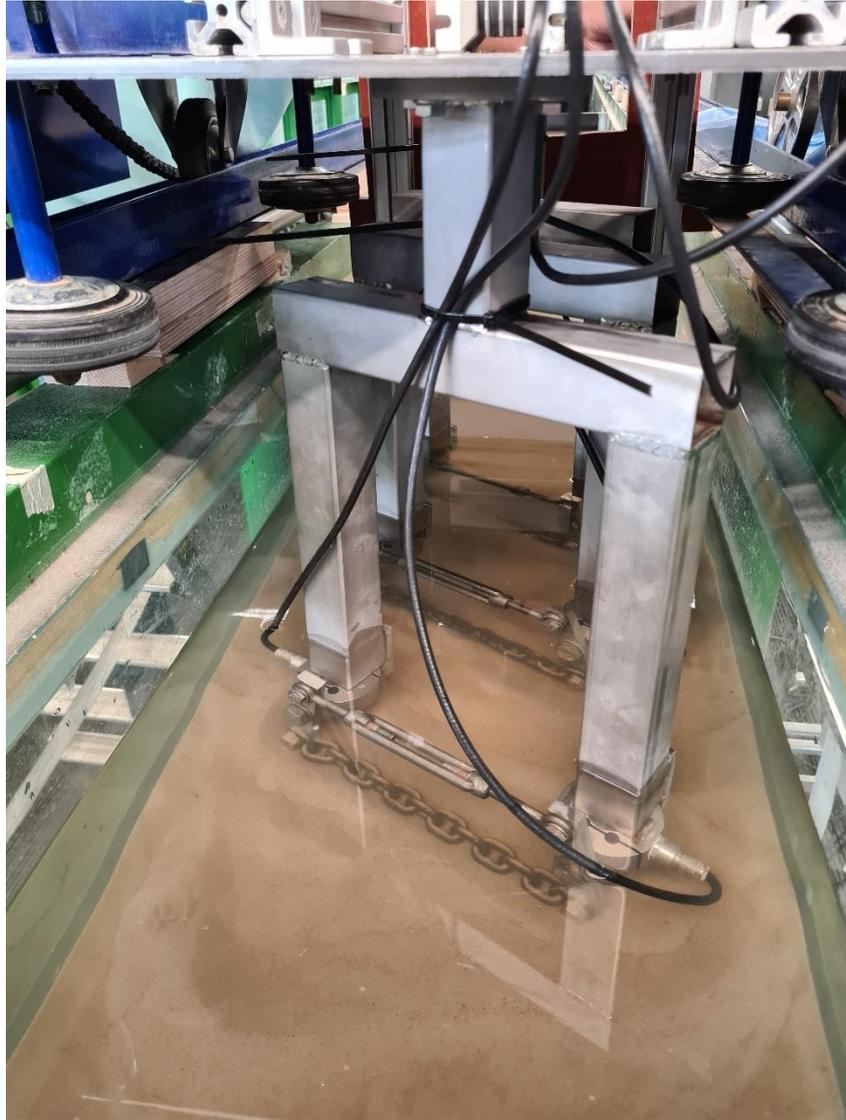
*Figure 43: Towing the chain at an angle of 60 degrees with respect to the towing direction*
