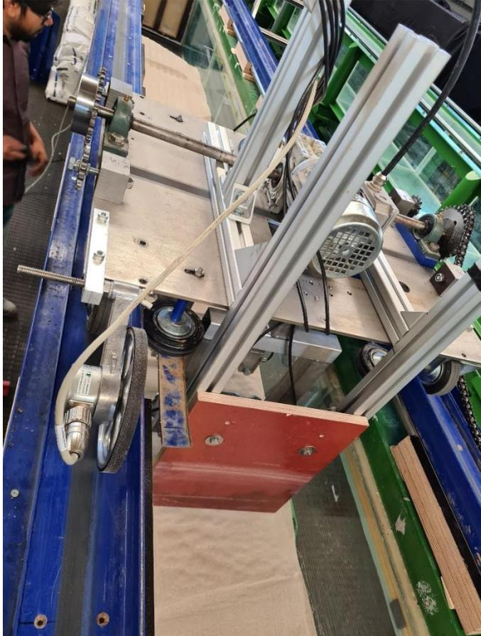
Figure 42: The wooden plate that is used to level the sandbed
