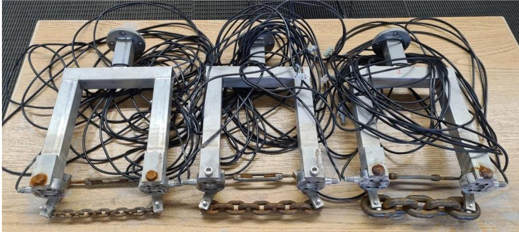
Figure 40: Three chain holders with different chain link diameters
