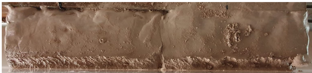
Figure 5.13: TC#02 : 17 mm nozzle at a 25 degree jetting angle with a stand-off distance of 5 cm. The forward velocity was 0.419 m/s and there was a flow rate of 119.4 l/min producing a jet velocity of 7.78 m/s.
