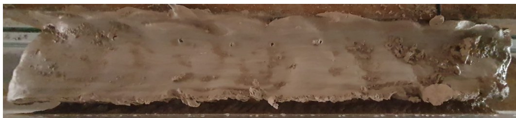
Figure 5.23: TC#12 : 17 mm nozzle at a 90 degree jetting angle with a stand-off distance of 10 cm. The forward velocity was 0.431 m/s and there was a flow rate of 174 l/min producing a jet velocity of 17.25 m/s.
