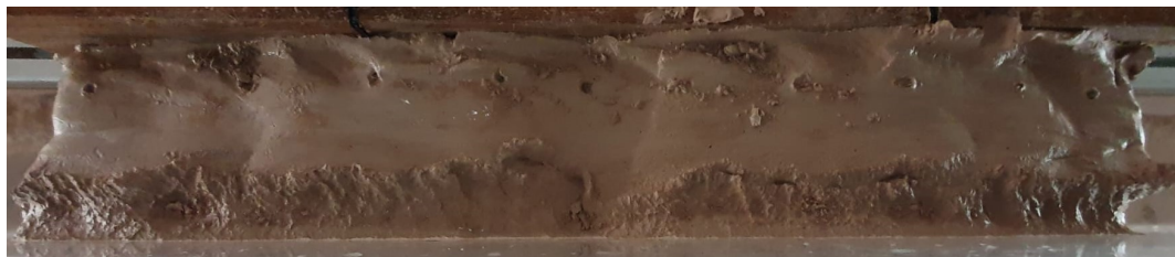
Figure 5.24: TC#13 : 20 mm nozzle at a 45 degree jetting angle with a stand-off distance of 10 cm. The forward velocity was 0.448 m/s and there was a flow rate of 185 l/min producing a jet velocity of 12.38 m/s.
