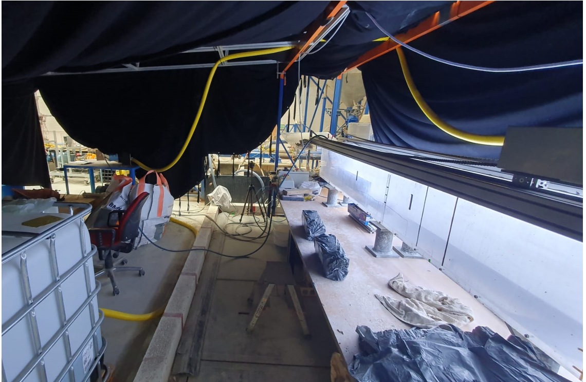
Figure 5.3: Overview of test set-up: This view allows one to see the work space I had available. The black cover around the work space was to minimize light glare on the cameras. The clay was back lit to increase the contrast and make the erosion process easier to see on camera.
