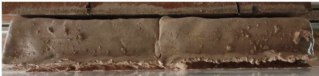
Figure 5.12: TC#01 : 17 mm nozzle at a 90 degree jetting angle with a stand-off distance of 5 cm. The forward velocity was 0.422 m/s and there was a flow rate of 120 l/min producing a jet velocity of 11.90 m/s.
