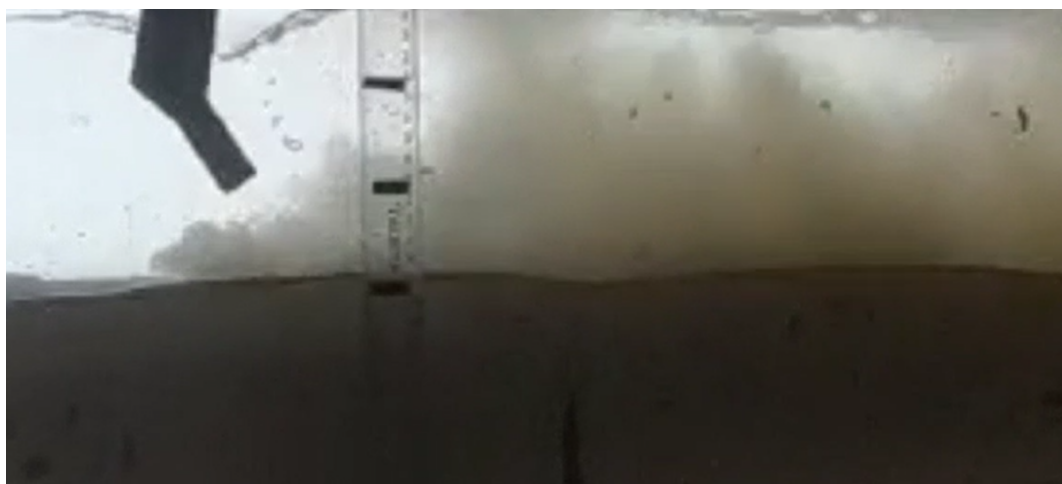
Figure 7.4: The sediment plume formed by a 12 mm water jet at 135^\circ (the jet is moving from right to left).
