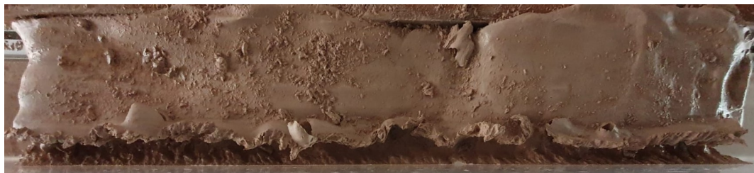
Figure 5.18: TC#07 : 17 mm nozzle at a 115 degree jetting angle with a stand-off distance of 5 cm. The forward velocity was 0.402 m/s and there was a flow rate of 126 l/min producing a jet velocity of 12.09 m/s.
