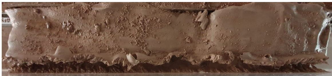
Figure 7.2: TC07-4: 17 mm nozzle angled at 115^\circ with a stand-off distance of 5 cm. The forward velocity was 0.402 m/s and there was a flow rate of 126 l/min.
