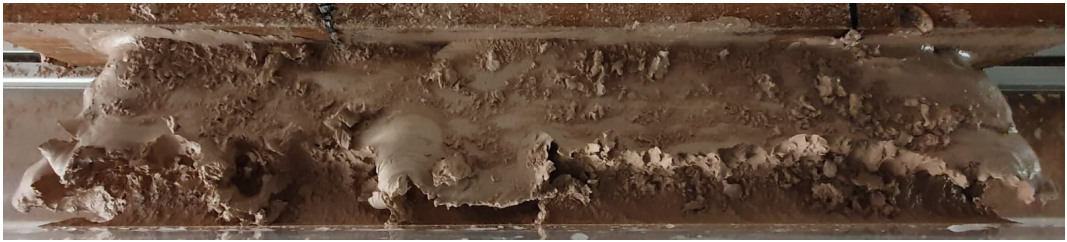
Figure 5.15: TC#04 : 17 mm nozzle at a 65 degree jetting angle with a stand-off distance of 5 cm. The forward velocity was 0.414 m/s and there was a flow rate of 126 l/min producing a jet velocity of 12.09 m/s.
