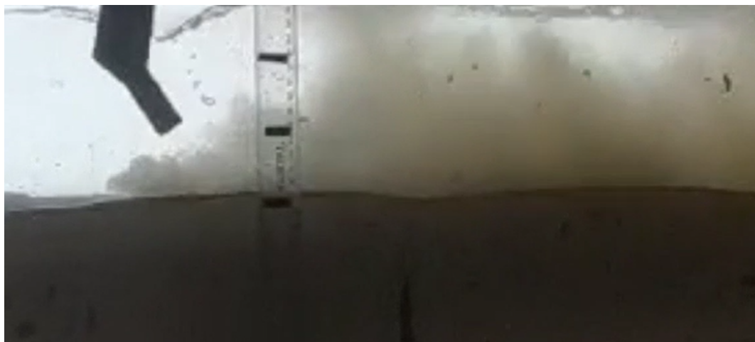
Figure 6.4: The sediment plume formed by a 12 mm water jet at 135^\circ (the jet is moving from right to left).
