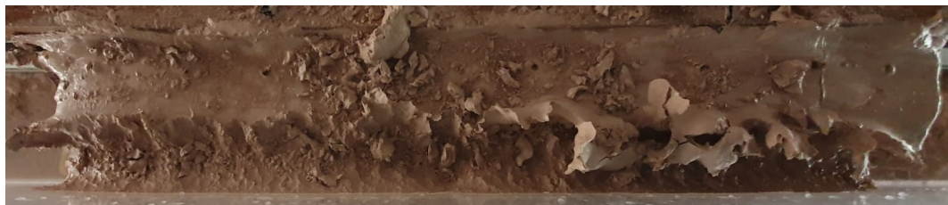
Figure 5.25: TC#14 : 20 mm nozzle at a 65 degree jetting angle with a stand-off distance of 10 cm. The forward velocity was 0.412 m/s and there was a flow rate of 181 l/min producing a jet velocity of 10.09 m/s.
