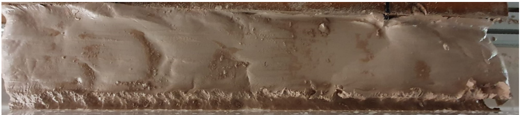
Figure 5.16: TC#05 : 17 mm nozzle at a 155 degree jetting angle with a stand-off distance of 5 cm. The forward velocity was 0.396 m/s and there was a flow rate of 120 l/min producing a jet velocity of 11.90 m/s.
