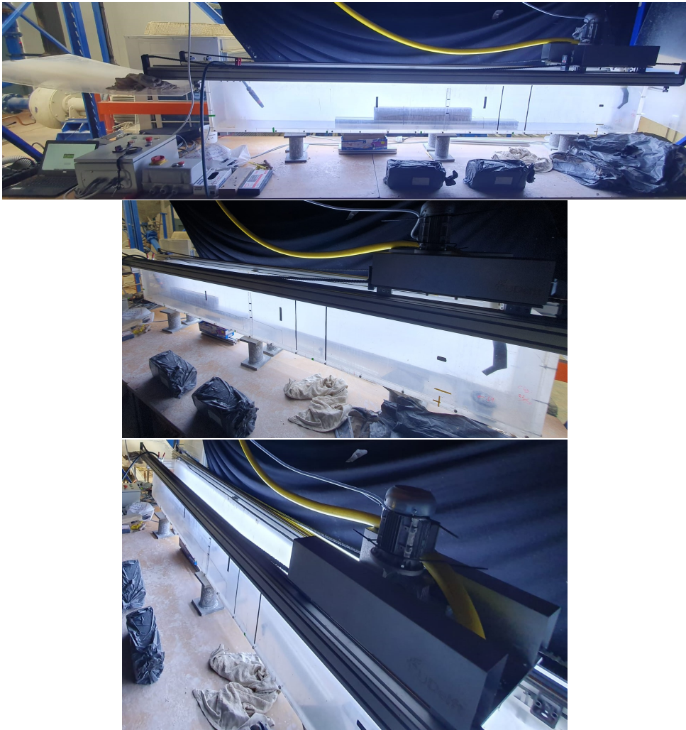
Figure 5.4: Flume test set-up: These images depict how the test rig was set-up and the overall appearance of the flume with the test rig mounted to it. There are three views available: front (top), angled (middle), and side (bottom).
