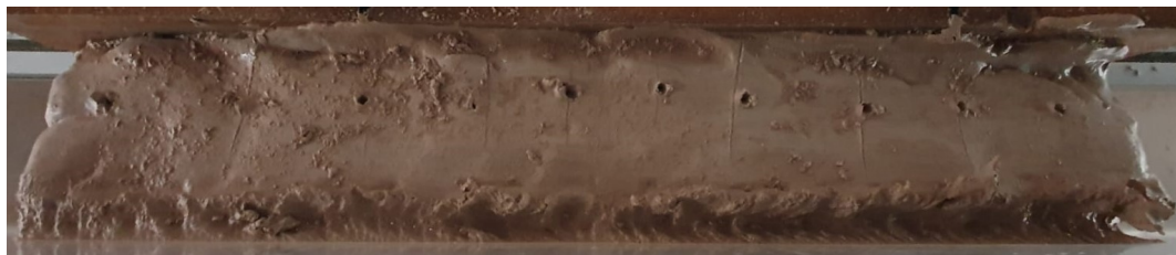
Figure 5.21: TC#10 : 12 mm nozzle at a 135 degree jetting angle with a stand-off distance of 5 cm. The forward velocity was 0.401 m/s and there was a flow rate of 81 l/min producing a jet velocity of 12.23 m/s.
