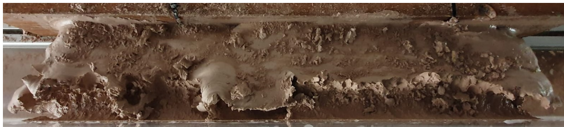
Figure 7.1: TC04-4: 17 mm nozzle angled at 65^\circ with a stand-off distance of 5 cm. The forward velocity was 0.414 m/s and there was a flow rate of 126 l/min.
