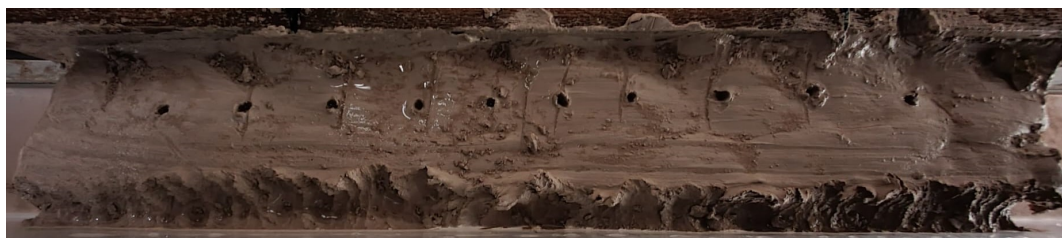
Figure 5.22: TC#11 : 20 mm nozzle at a 135 degree jetting angle with a stand-off distance of 5 cm. The forward velocity was 0.428 m/s and there was a flow rate of 177 l/min producing a jet velocity of 11.85 m/s.
