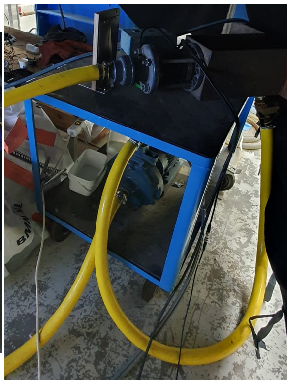
Figure 5.5: Pump test set-up: Hoses (yellow) were connected from the water tank (left) to the water pump (right) which was then routed from the water pump to the flow meter. The hose was then connected from flow meter to the nozzle and testing rig. This figure shows the blue cart used to hold the water pump (right, bottom) and the flow meter (right, top).
