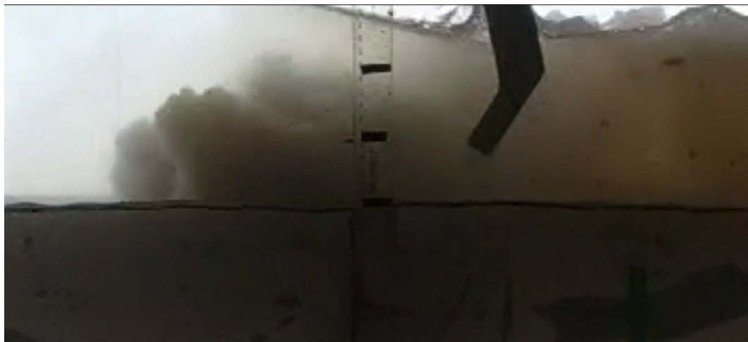
Figure 7.3: The sediment plume formed by a 17 mm water jet at 45^\circ (the jet is moving from right to left).
