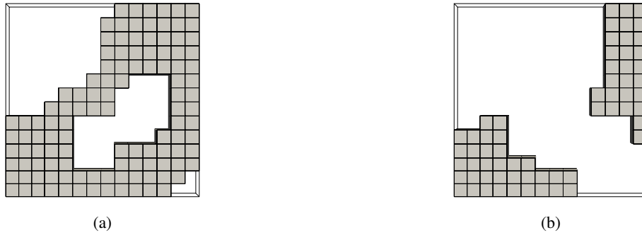
Figure 7: Elements used in the online phase in the two-dimensional strain localization problem: (a) DEIM –brown line in Figure 5a; (b) LDEIM –brown line in Figure 6a.
