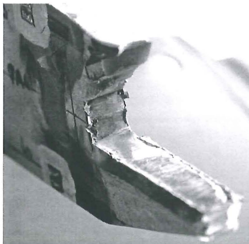
Figures 53.15 to 53.18: Several detailed perspectives of the failed weld.
