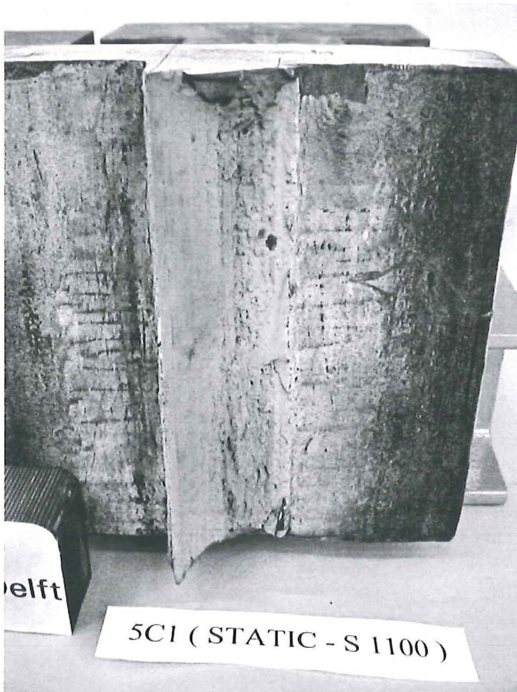
Figure 5C1-15c: Observed failure in the weld
