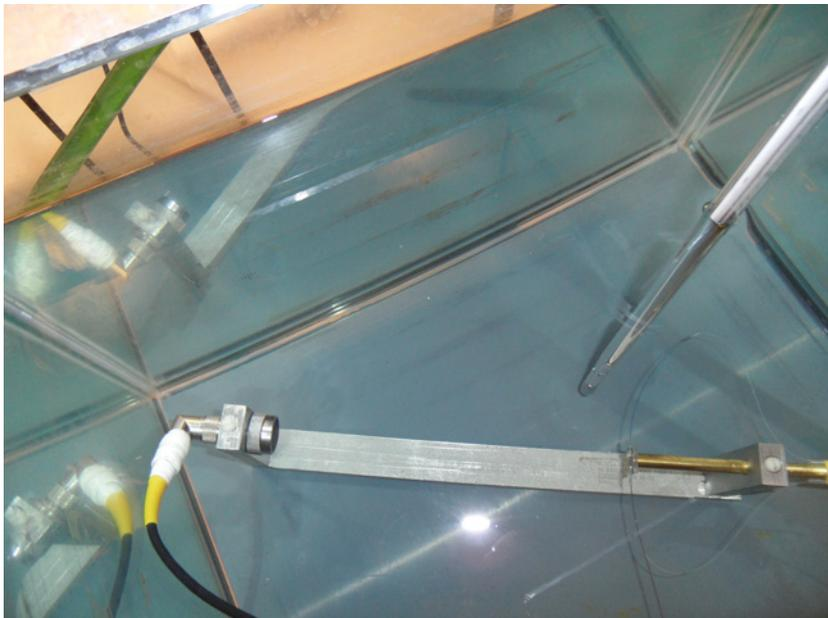
**Figure C.3:** Top-view of the water basin with the U-frame with the photonic chip microphone (right) and traditional ultrasound transducer (left). The pole sticking from above into the water is a thermometer.
