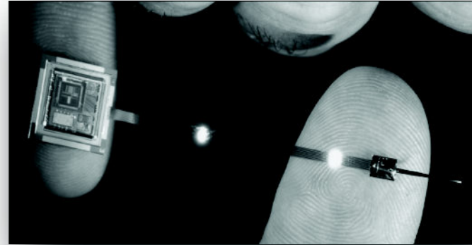
Source: A 32-Site 4-Channel High-Density Electrode Array for a Cochlear Prosthesis, Pamela T. Bhatti, Kensall D. Wise
