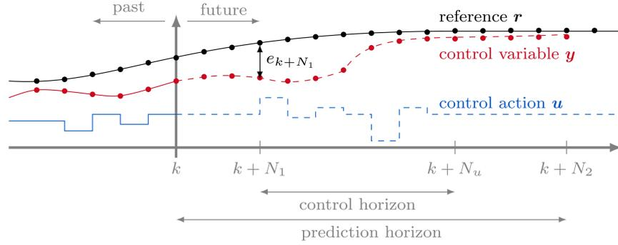
**Figure 5-1:** Function principle of a model-based predictive controller, with horizons  $N_1$ ,  $N_2$ ,  $N_u$  [23]
