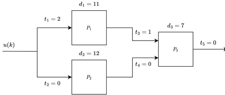
**Figure 5-2:** A simple manufacturing system
