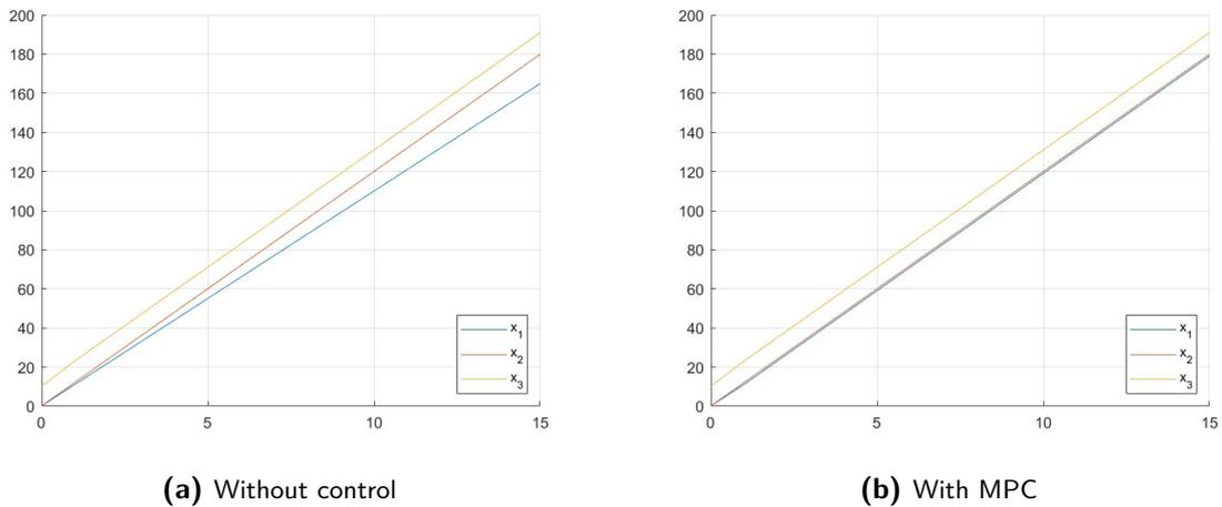
**Figure 5-3:** Simulation of max-plus-linear manufacturing unit, with initial state  $x_0 = [0, 0, 10]^T$ .
