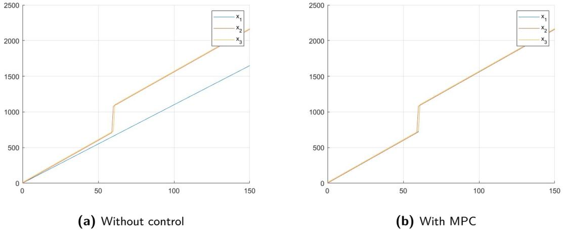
**Figure 5-4:** Simulation of max-plus-linear manufacturing unit with disturbance, with initial state  $x_0 = [0, 0, 10]^T$ .
