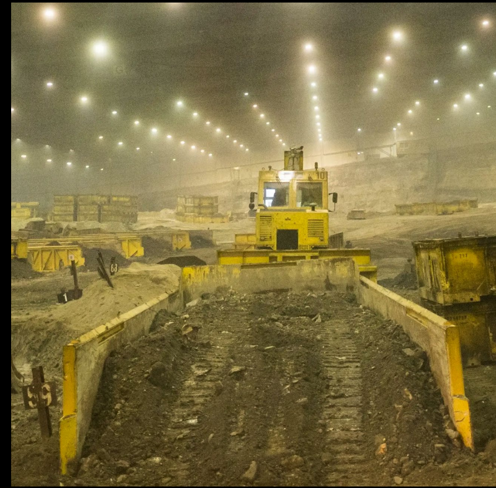
Sondermülldeponie Kölliken Photo of the explosion-proof vehicle used in the site's decontamination efforts, 2007-2015
