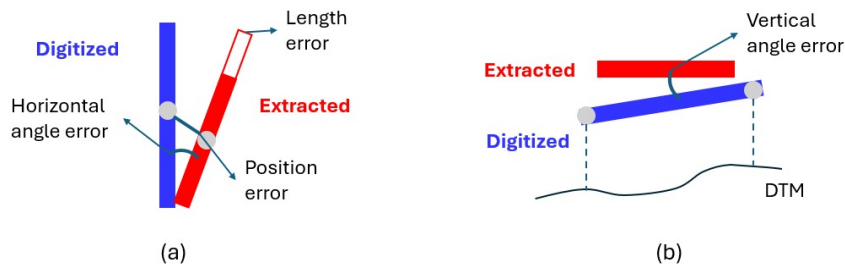
Figure 3.17: Aspects for evaluating line accuracy. Blue lines represented manually digitised lines, red lines represented automatically extracted lines. (a) Top view. (b) Side view
