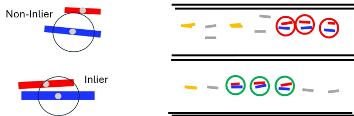
Figure 3.20: Illustration of RANSAC inliers evaluation. Blue lines represent road markings in the reference dataset, red lines represent road markings in the target dataset, and green-circled pairs are counted as inliers, red-circled pairs are counted as non-inliers
