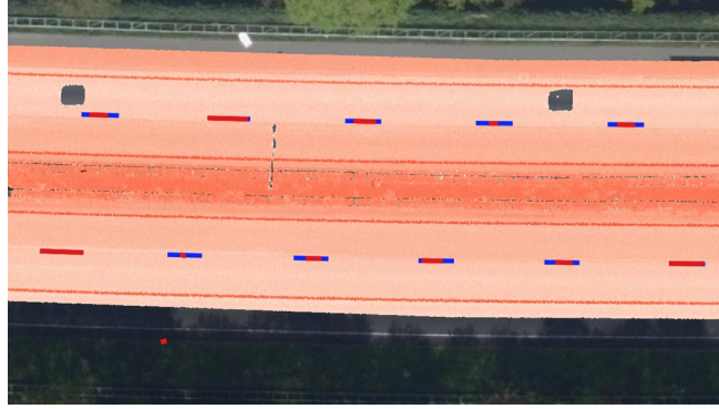
Figure 4.12: Sample of road markings detected in Prorail 2023 point cloud. Blue lines represent manually digitised road markings. Red lines represent automatically extracted road markings.
