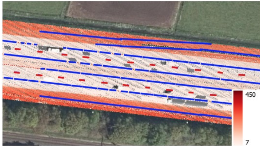
Figure 4.7: Detection error in AHN3 point cloud. Blue lines represent automatically extracted road marks, red lines represent manually digitised road marks (as a reference for detection accuracy measurement)
