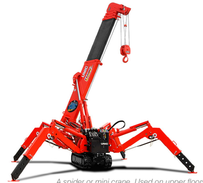
A spider or mini crane. Used on upper floors.
