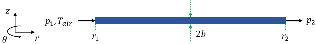
Figure 3.3: Schematic representation of the axisymmetric air layer geometry.
