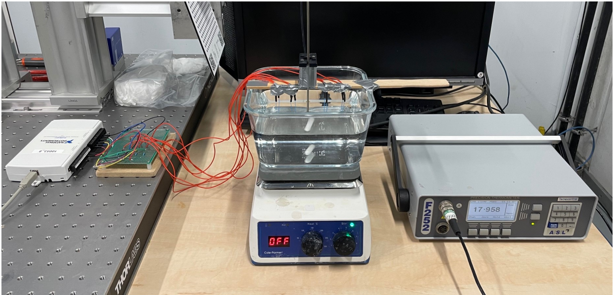
Figure F.7: Calibration setup used for the thermistors.
