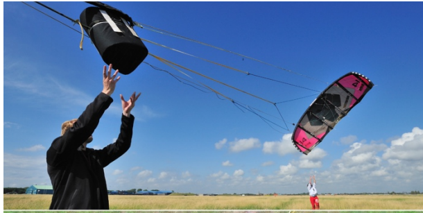
Figure 4. Kite Control Unit and bridle system during launch (Photo: Max Dereta)
