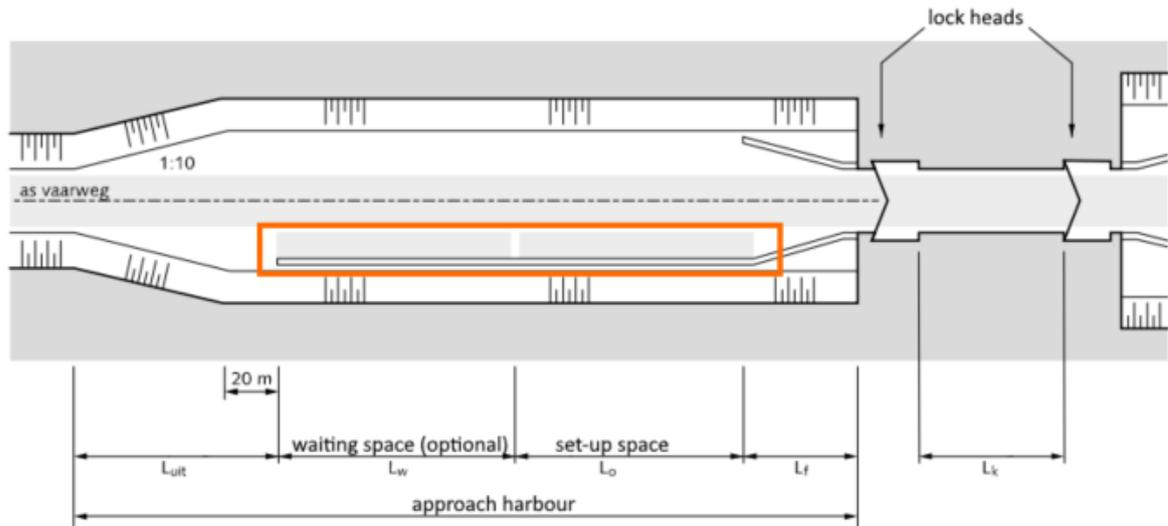
Figure 1.2: Schematic drawing of a lock with approach harbour. Together, the waiting space and set-up space, which are framed, form the waiting places and are thus the area of interest, adapted from (RWS WVL, 2020)
