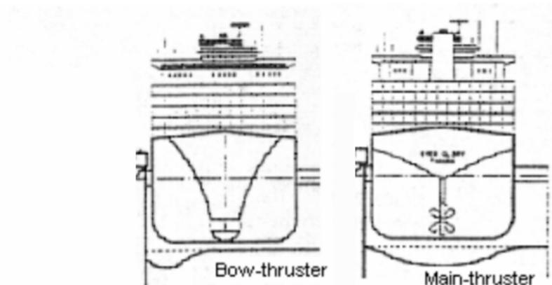
Figure 2.3: Location of scour from bow thruster (left) and main propeller (right) (Roubos & Verhagen, 2007)
