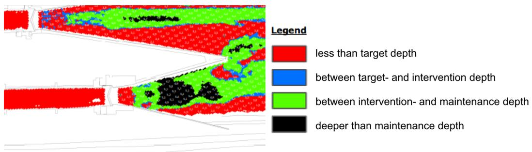
Figure 3.22: Multibeam drawing of Belfeld, translated from RWS Dienst Infrastructuur and Iv-Infra B.V. (2010)
