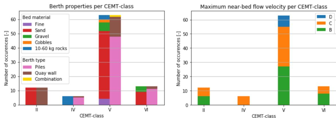
Figure 5.2: Distribution of berth properties (left) and near-bed flow velocities (right) of waiting places per CEMT-class
