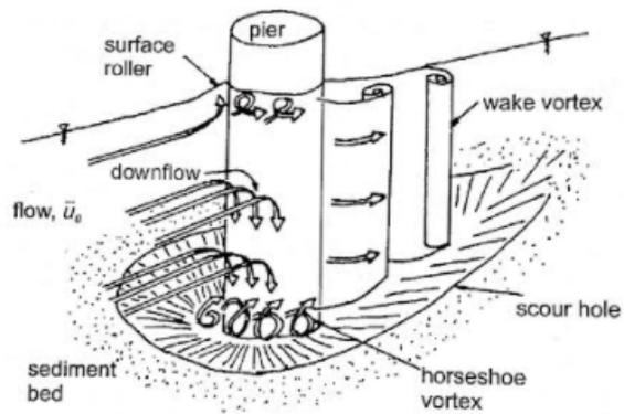
Figure 2.6: Scour along a pile (Breusers & Raudkivi, 1991)
