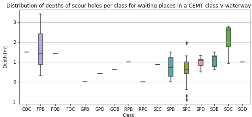
Figure 5.9: Distribution of depths of scour holes per class for waiting places in a CEMT-class V waterway
