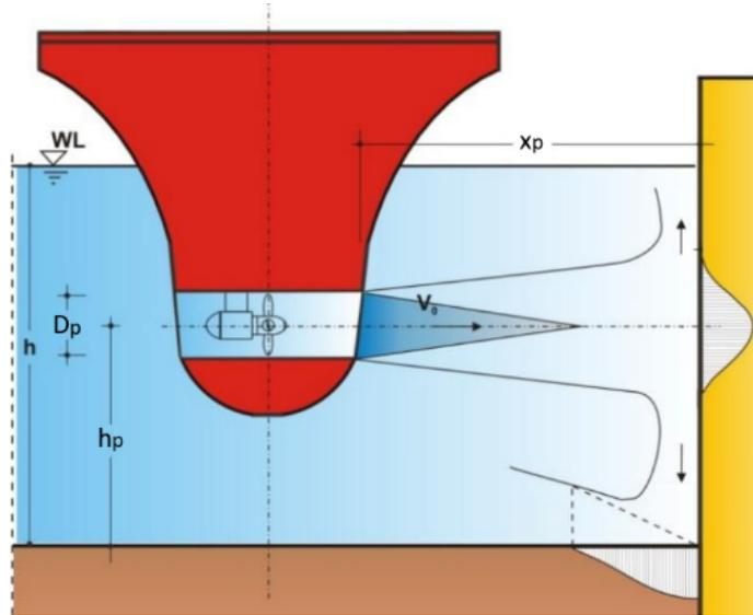
Figure 2.4: Scour of bed by bow thruster when sailing away in order to enter the lock, adapted from PIANC (2015)
