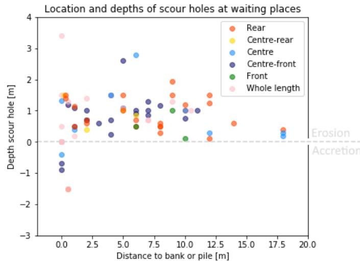
Figure 3.23: Visualisation of the location and depth of scour holes, where a negative scour hole depth equals accretion and a positive depth erosion
