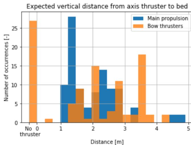
Figure 3.8: Histogram with 20 bins of the vertical distances between the axis of the propeller and the bed
