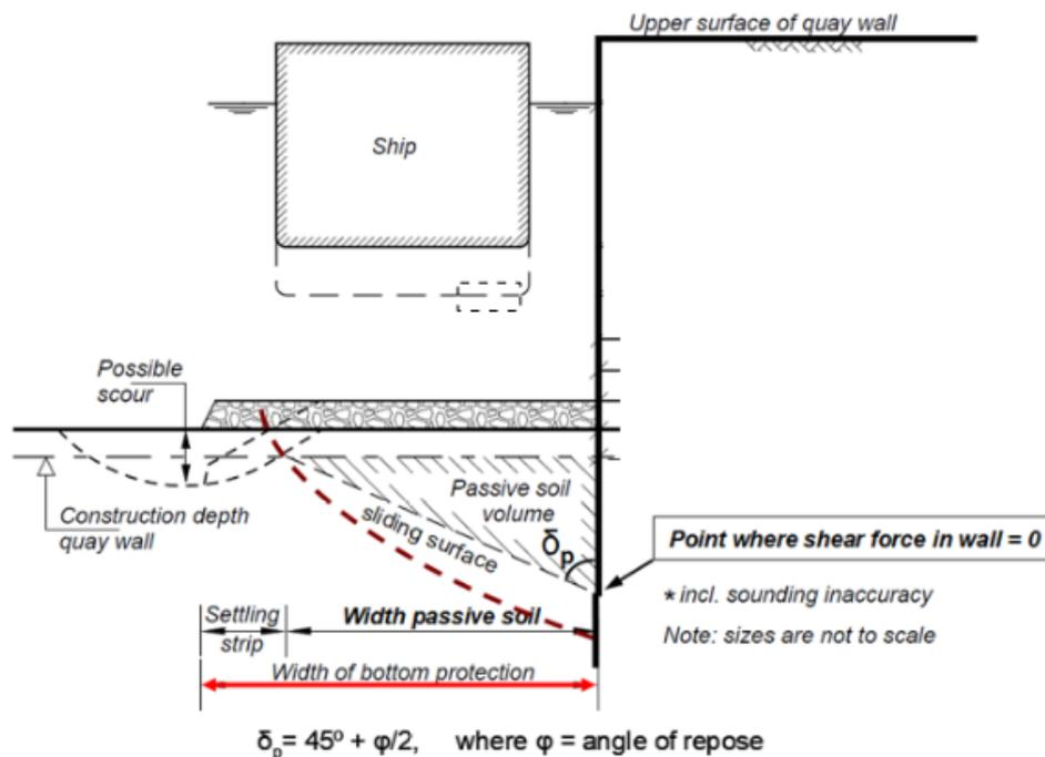
Figure 2.13: Passive soil wedge and width of the bed protection, adapted from Tipton and Krause (2013)
