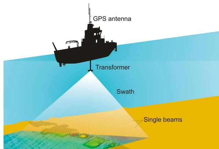
Figure 3.19: Scanning with Multibeam Bathymetry (Wessex Archeology, 2010)
