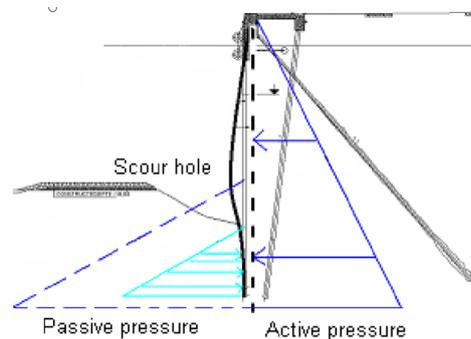
Figure 1.1: Collapse of a quay wall after a scour hole is created, adapted from Roubos and Verhagen (2007)
