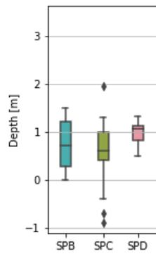
(a) Distribution of scour depths for increasing  $V_{bed}$
