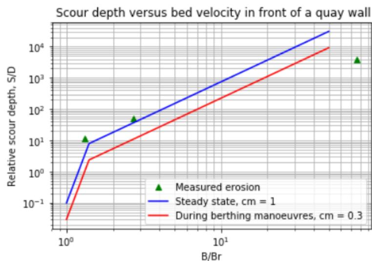
Figure 6.2: Measured erosion of this thesis compared to empirical formulas based on measurements of Römisch (2006)
