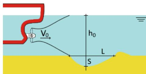
Figure 2.9: Scour due to a horizontal propeller
