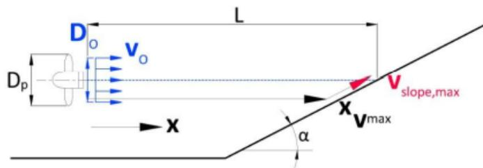
Figure 2.5: Transverse thruster jet above a slope (PIANC, 2015)
