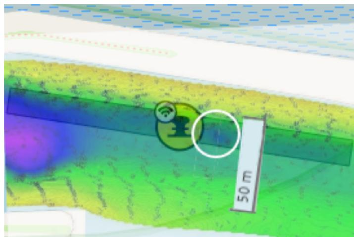
Figure 6.1: Snapshot from Vaarweginformatie.nl of outer waiting place the Zandkreek lock with the multibeam drawing placed on top of it. The white circle shows the location of the scour hole. Adapted from RWS Dienst VenW (2022) and RWS Dienst Infrastructuur (2013)
