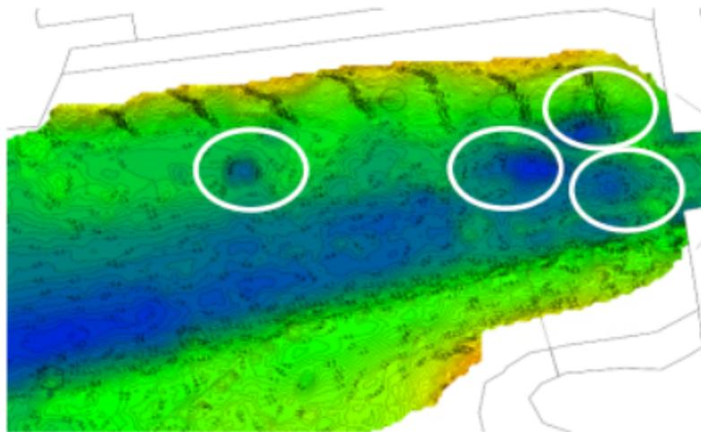
Figure 3.20: Multibeam drawing of the bed at the Zandkreek lock, where several scour holes are pointed out with white circles. Adapted from RWS Dienst Infrastructuur (2013)
