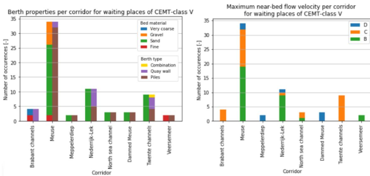
Figure 5.17: Distribution of berth properties (left) and near-bed flow velocities (right) of waiting places per corridor for waiting places in a CEMT-class V waterway
