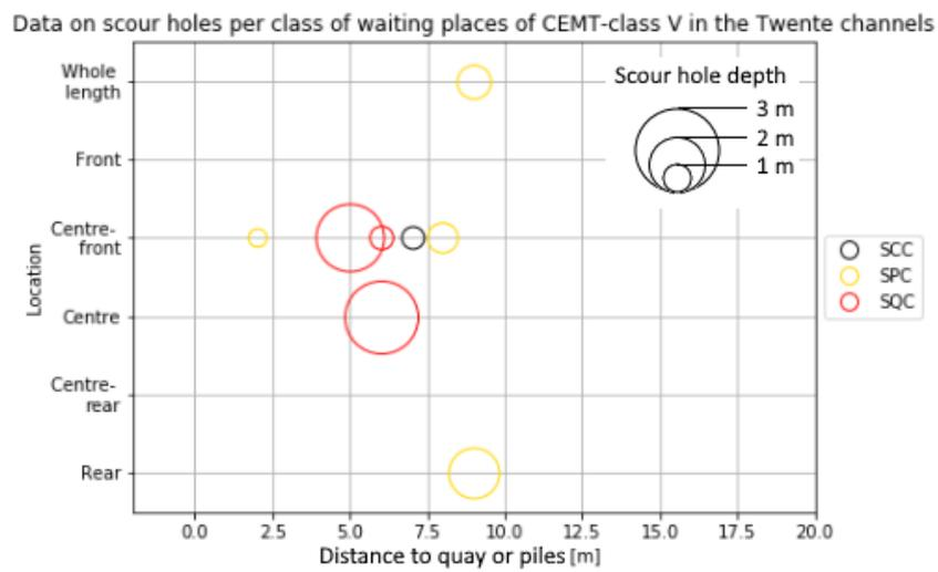
Figure 5.26: Location and depth of scour holes per class of waiting places in the Twente channels
