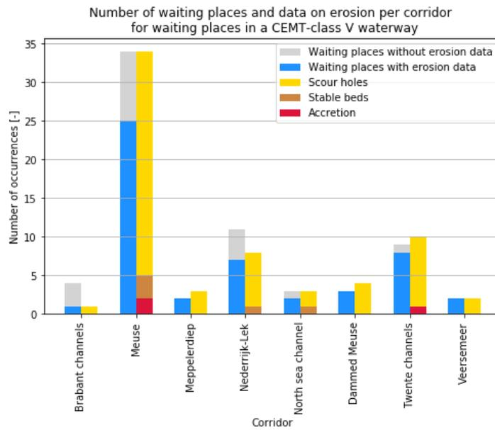
Figure 5.16: Number of waiting places, availability of erosion data, and scour holes per corridor for waiting places in a CEMT-class V waterway
