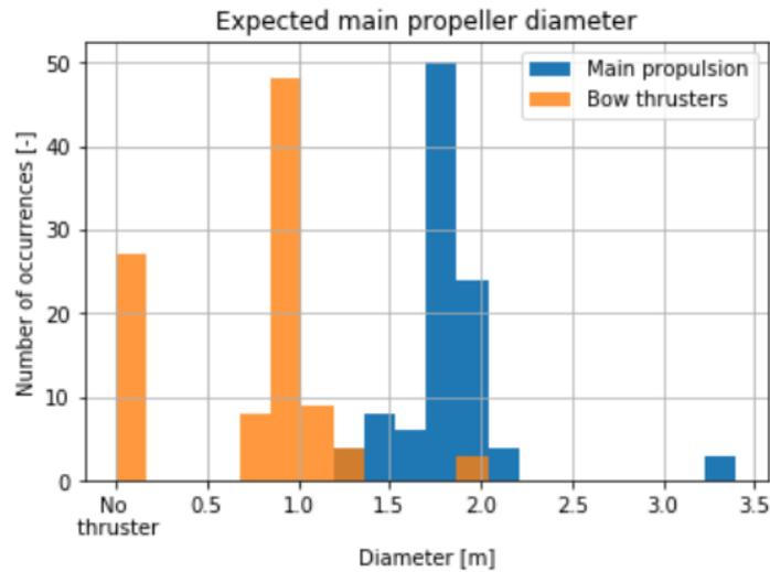
Figure 3.7: Histogram with 20 bins of the propeller diameters of both the main propellers and bow thrusters of the design vessel
