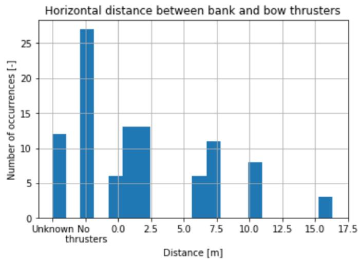
Figure 3.9: Histogram with 20 bins of the horizontal distances between the axis of the bow thruster and the bank
