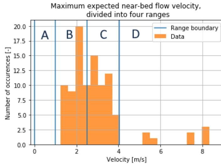
Figure 4.2: Range boundaries for the maximum near-bed flow velocity
