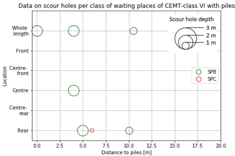
Figure 5.14: Location and depth of scour holes per class of waiting places in CEMT-class VI waterways for waiting places with piles
