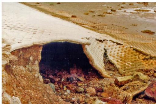
Figure 2.11: Failed concrete lining (Heibaum & Trentmann, 2010)
