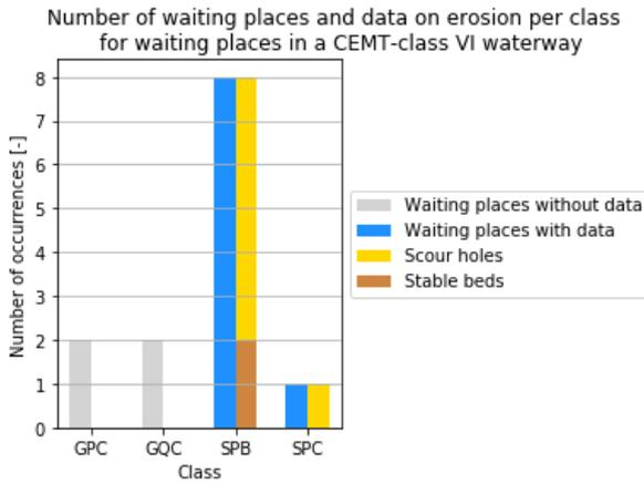
Figure 5.12: Number of waiting places, availability of erosion data, and scour holes in each class for waiting places in a CEMT-class VI waterway
