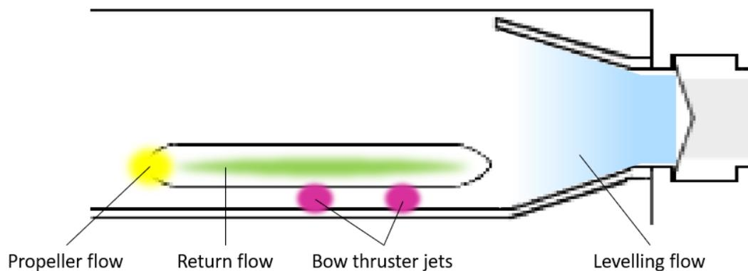
Figure 2.1: Locations of different types of loads acting on the bed protection for a ship with two bow thrusters
