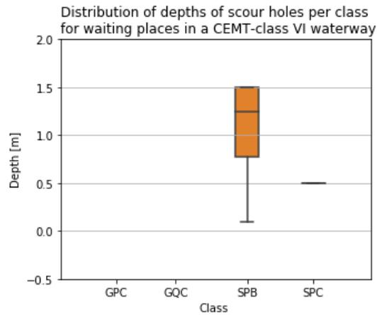
Figure 5.13: Distribution of depths of scour holes per class for waiting places in a CEMT-class VI waterway
