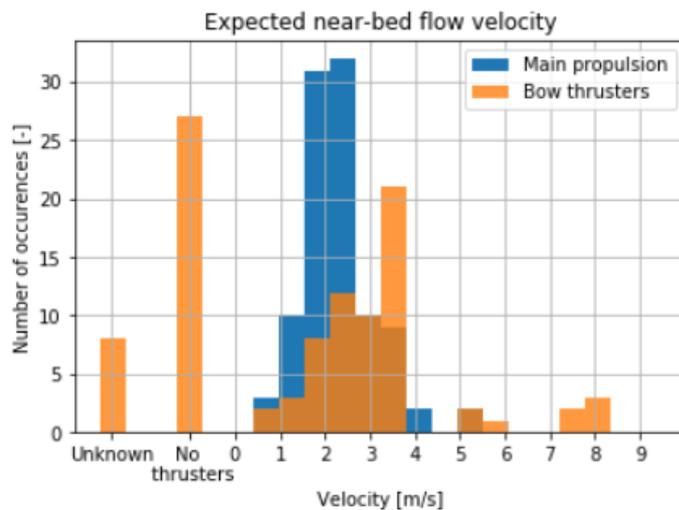
Figure 3.18: Histogram with 20 bins of the expected near-bed flow velocities caused by either the main propulsion system or bow thrusters
