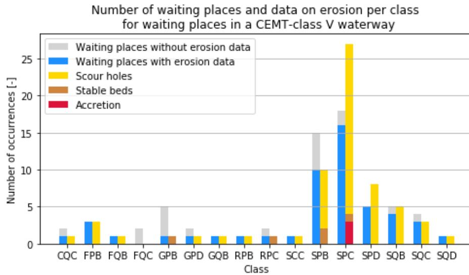
Figure 5.8: Number of waiting places and scour holes in each class for waiting places in a CEMT-class V waterway
