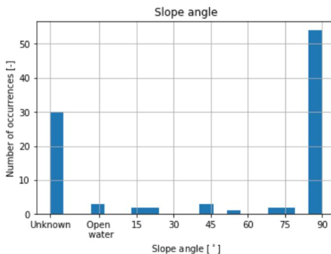
Figure 3.14: Histogram with 20 bins of the angle of the slope of the banks at the waiting places
