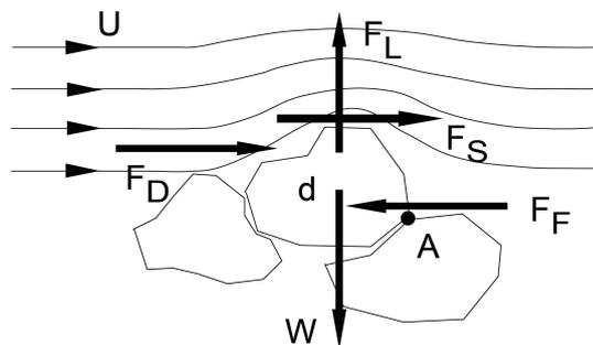
Figure 2.10: Schematic of forces on a grain by flow (Schierneck, 2019)
