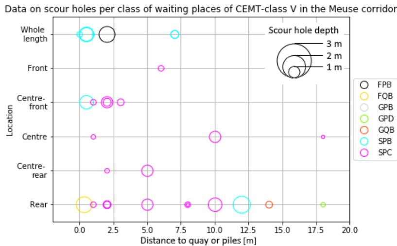
Figure 5.20: Location and depth of scour holes per class of waiting places in the Meuse
