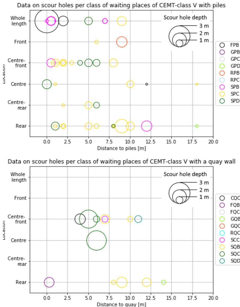
Figure 5.11: Location and depth of scour holes per class of waiting places in CEMT-class V waterways for waiting places with piles (top) and quay walls (bottom)
