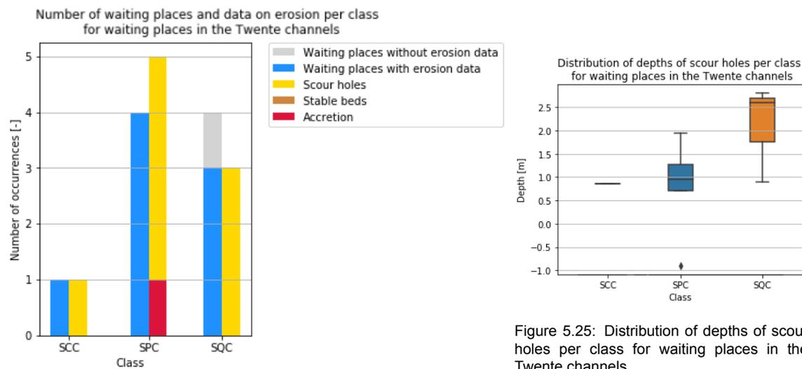
Figure 5.25: Distribution of depths of scour holes per class for waiting places in the Twente channels
