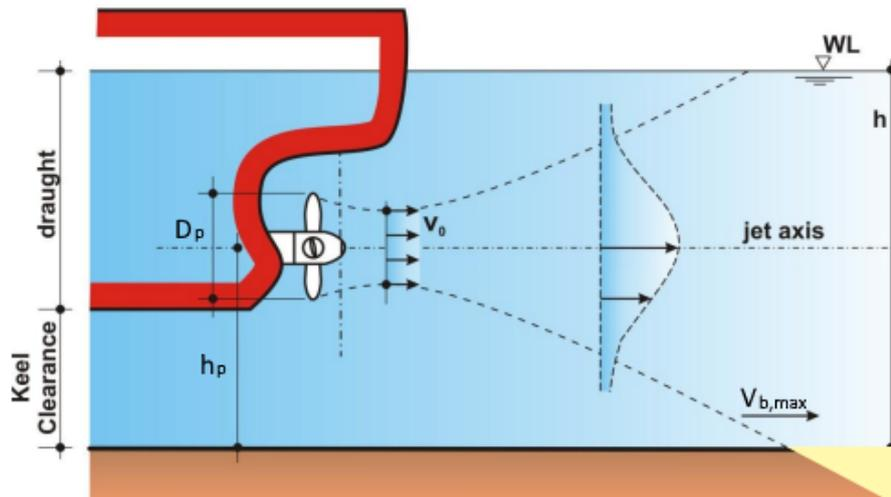
Figure 2.2: Scour of bed by main propulsion system (adapted from PIANC (2015))
