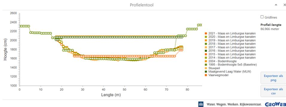
Figure 3.16: Cross section of waterway at location as shown in Figure 3.15 (Rijkswaterstaat & GeoWeb, 2022)
