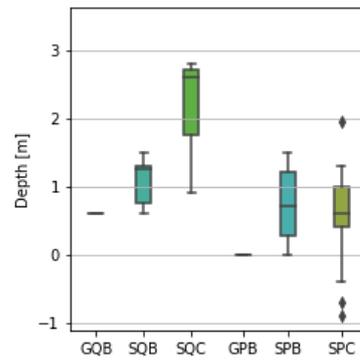
(b) Distribution of scour depths for three sets of classes where only the berth type (quay vs. piles) differs
