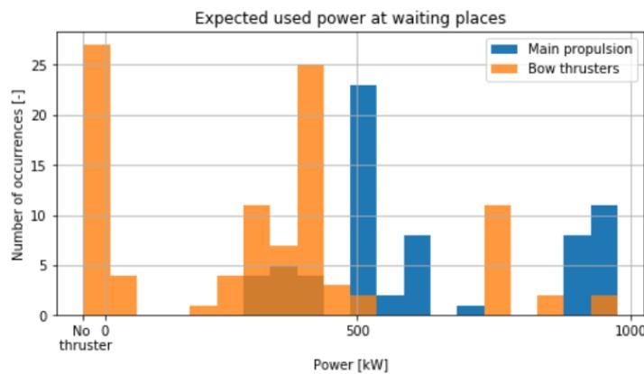
Figure 3.6: Histogram with 20 bins of the used power per propeller of both the main propellers and bow thrusters at waiting places
