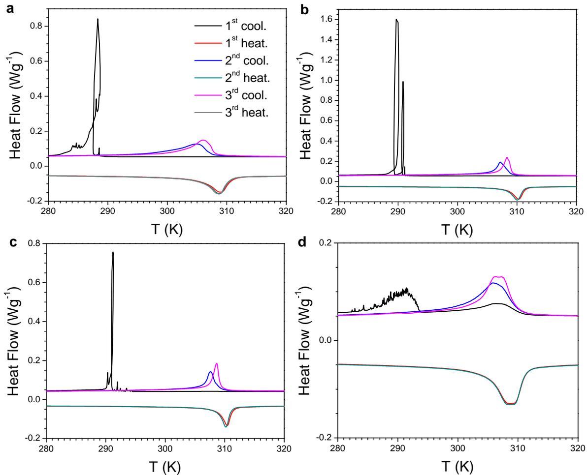
**Fig. 1.** Heat flow upon successive cooling and heating (at  $5 \text{ K min}^{-1}$ ) across the first-order magnetic transition of  $\text{Mn}_{1.23}\text{Fe}_{0.72}\text{P}_{0.48}\text{Si}_{0.52}$  in different shapes: (a) large bulk piece (mass = 110.1 mg), (b) an intermediate size bulk piece (35.5 mg), (c) crushed powder having particle size  $>75 \mu\text{m}$ , and (d) powder having particle size  $<30 \mu\text{m}$ .
