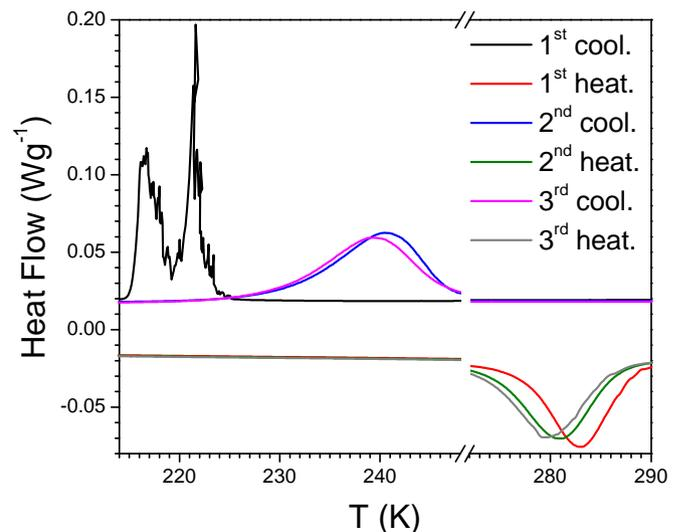
**Fig. 3.** Heat flow upon successive cooling and heating (measured at  $2 \text{ Kmin}^{-1}$ ) across the first-order magnetic transition of  $\text{MnFe}_{0.95}\text{P}_{0.62}\text{Si}_{0.34}\text{B}_{0.04}$  (bulk piece of 108.0 mg).
