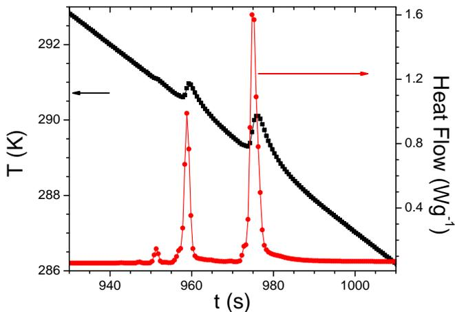
**Fig. 2.** Time dependence of the sample pan temperature and heat flow during the first cooling of an as-prepared  $\text{Mn}_{1.23}\text{Fe}_{0.72}\text{P}_{0.48}\text{Si}_{0.52}$  sample (intermediate size bulk piece, 35.5 mg, Fig. 1(b)).
