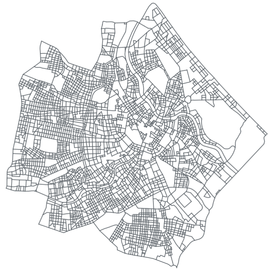
Fig. 6. Constrained airspace structure extracted from the street network of the city centre of Vienna.
