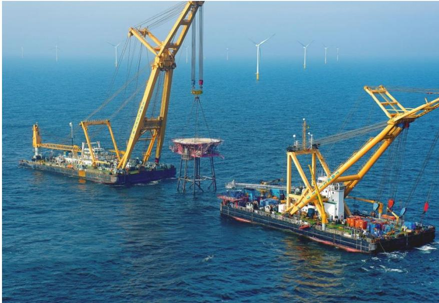
Figure 1-8 Boskalis' floating sheerleg vessels Taklift 4 and Taklift 7
