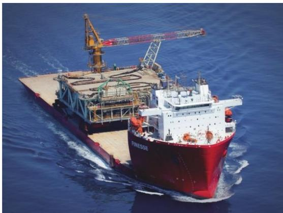
Figure 1-1 F-class Semi-Submersible Heavy Transport Vessel Finesse
