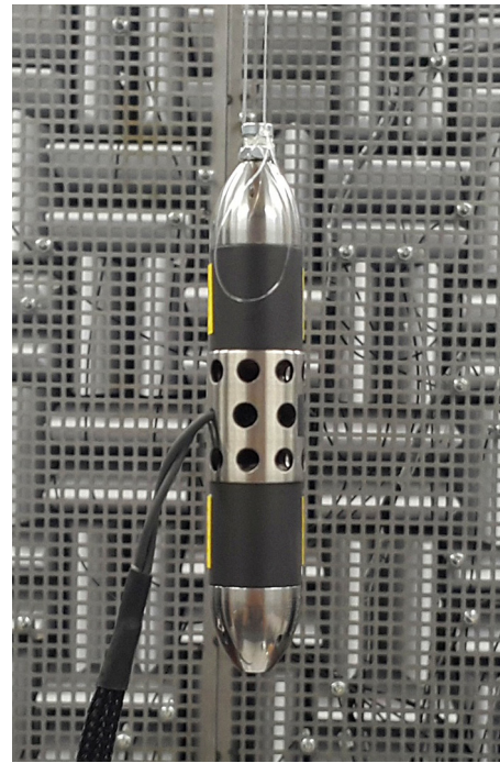
FIG. 5. (Color online) Customized miniature sound source (omnidirectional in the azimuthal plane).
