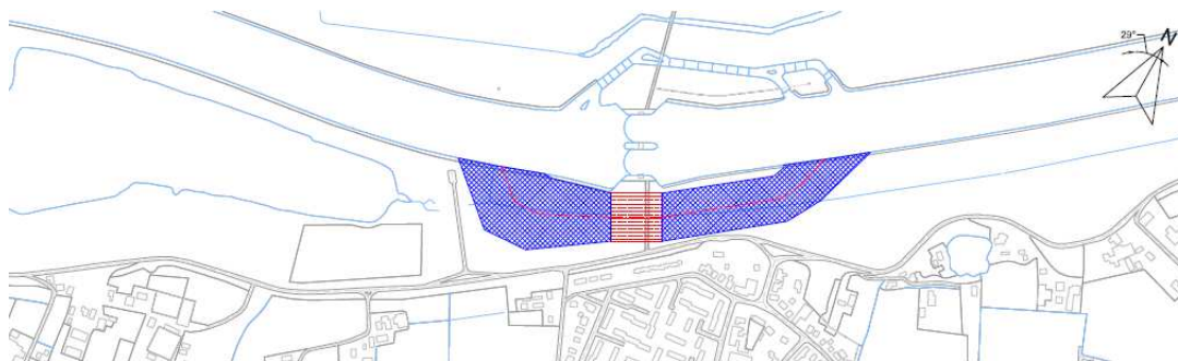
Figure 46 - Hydro-power-scheme-variant 1 - Sketch of bay power-plant south of the weir at Driel – see Appendix 14 .
