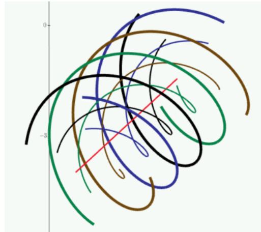
Figure 21 – 3D image of reconstructed geometry of the blade edge and connection to central axis of the Dommelstroom turbine and a picture for reference
