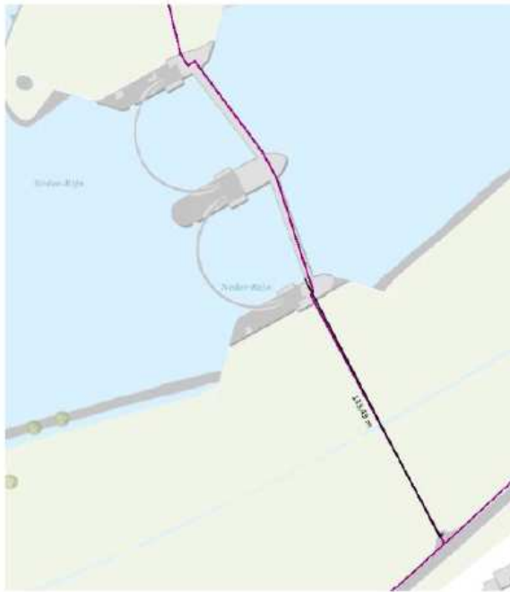
Figure 42 - Location of power-cables to which any hydro-power near the weir can be connected. Medium Voltage cable runs, through the weir. From Liandon: [33]
