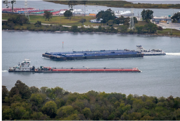
Figure 3.1: Articulated Tug and Barge combinations (ATBs) on the Houston Ship Channel seen from the San Jacinto Battleground Monument.
