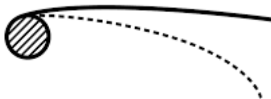
Figure 5.4: Sketch of a Leading Edge Inflatable tube airfoil
