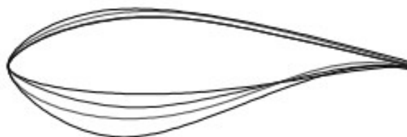
Figure 2.5: Overlap of DU Wind Turbine airfoils from Timmer and van Rooij[10].
