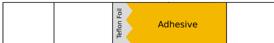
Figure 3.4: Triangular disbond front, adjusted from[20]
