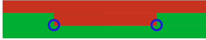
Figure 3.10: Example disbond front, the green area is bonded and the red area has failed
