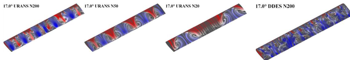
Figure 2.19: Wall shear stress stall cell observations for URANS and DDES with different grid resolutions, figure from Manni et al. (2016)
