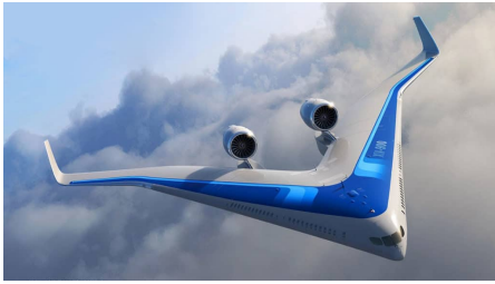
Figure 3.4: The Flying V configuration. Left: render view. Right: FD initial dimensions [33].
