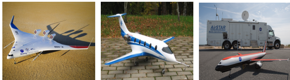
Figure 1.4: Left: X-48B (NASA) 8.5% geometrically scaled SM . Center: Raven (University of Linköping) 13.8% geometrically and Froude's scaled SM . Right: AirSTAR (Air-Force Research Laboratory USA) 5.5% geometrically scaled tube-wing SM with Froude's scaling.
