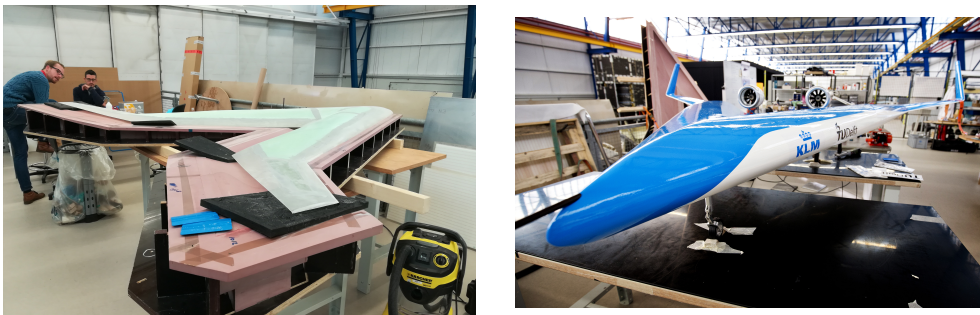
Figure 6.1: Left: Flying V model under construction at the manufacturing lab of the TUD. Right: Real-built Flying V model.
