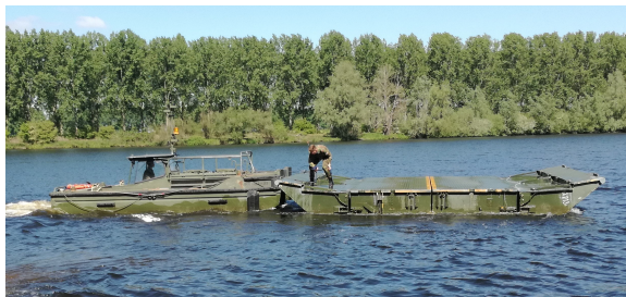
Figure 1.2: BresDefender pontoon connected to a boat for transportation
