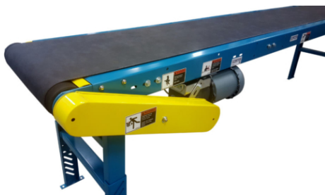
(a) Belt conveyor
