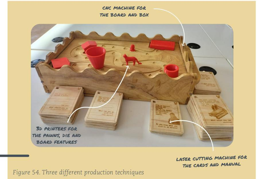
Figure 54. Three different production techniques
