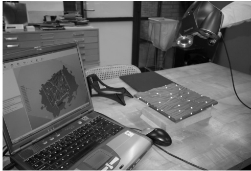
Figure 4 WAD-tile project: 3D scan experiments and final tile prototype on display
