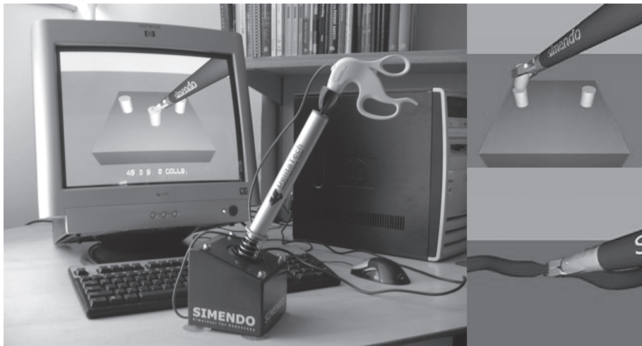
Figure 1. Left: the SIMENDO connected to the PC via USB-port. Right: two exercises: piling up of cylinders and clipping of a vessel
