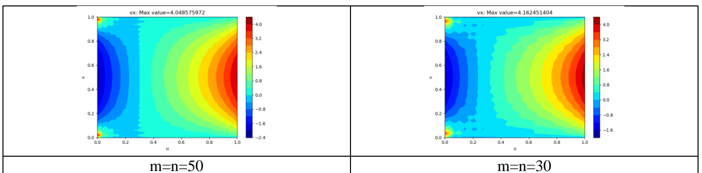
Figure 106: Test SC2 shear force v_x results ( m=n= 30, 50 )
