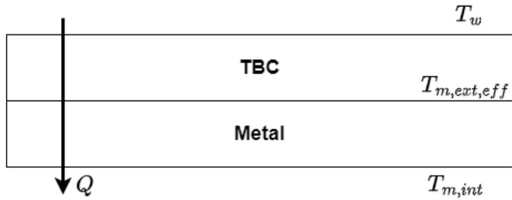
Figure 3.12: Model of the heat transfer process through the thermal barrier coating and substrate blade metal
