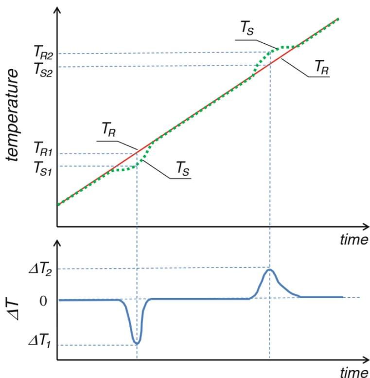
Figure 3. a general DTA temperature-time curve. (Kośny, 2015)
