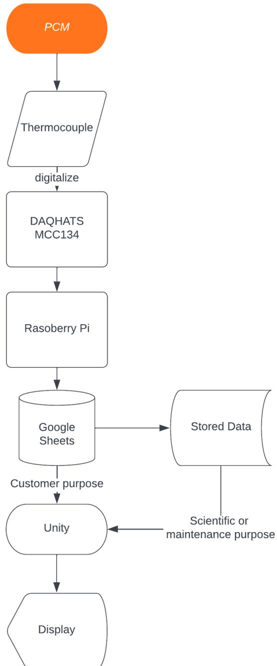
Figure 47. Dataflow from PCM to Display.
