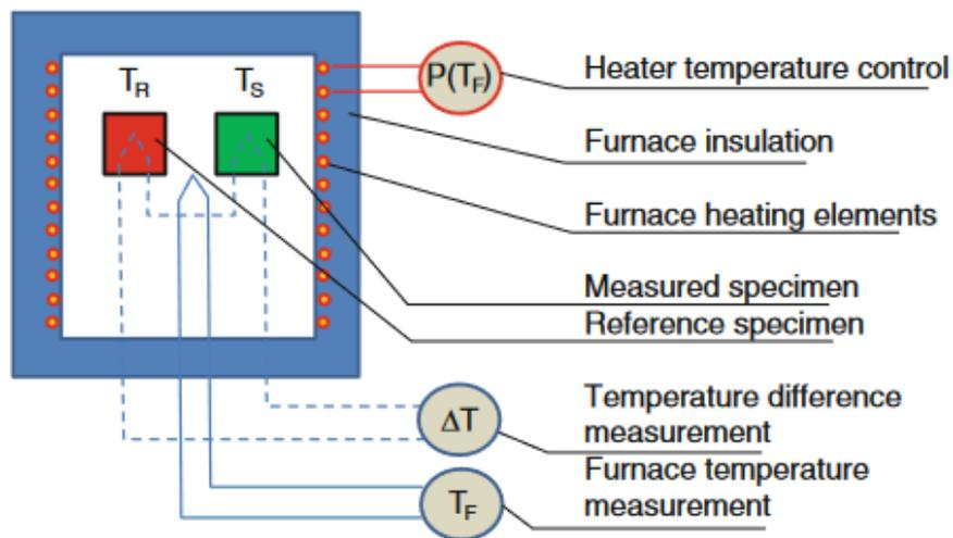
Figure 2. typical setup for a DTA. (Kośny, 2015)
