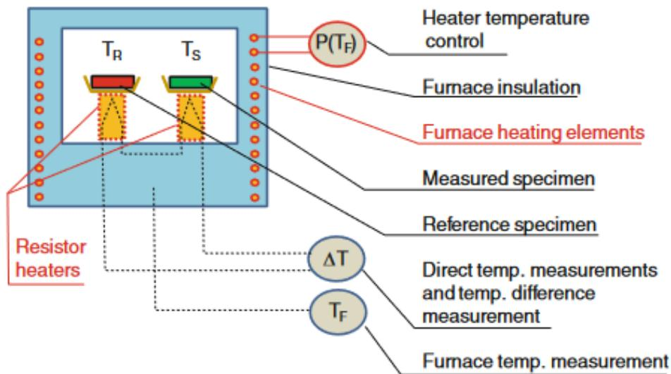
Figure 4. typical setup for a DSC. Kośny (2015)
