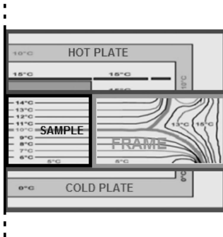
Figure 9. a schematic section of a dynamic guarded hot plate method.(Pomianowski et al., 2014)
