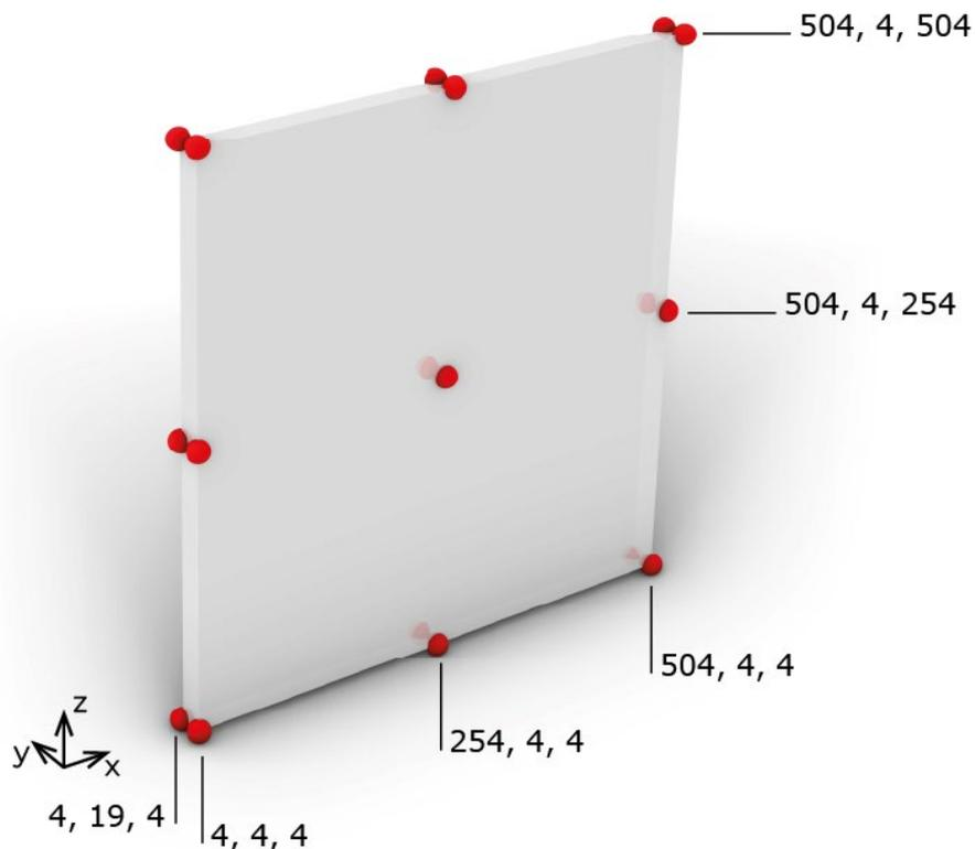
Figure 1914. Location of the temperature probes
