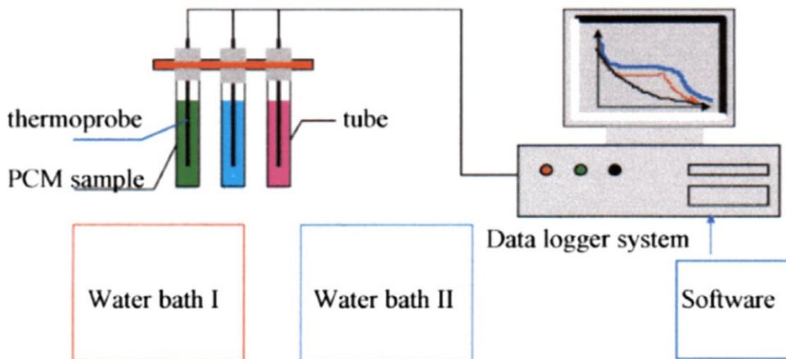
Figure 6. The first T-history setup.(Yinping et al., 1999)
