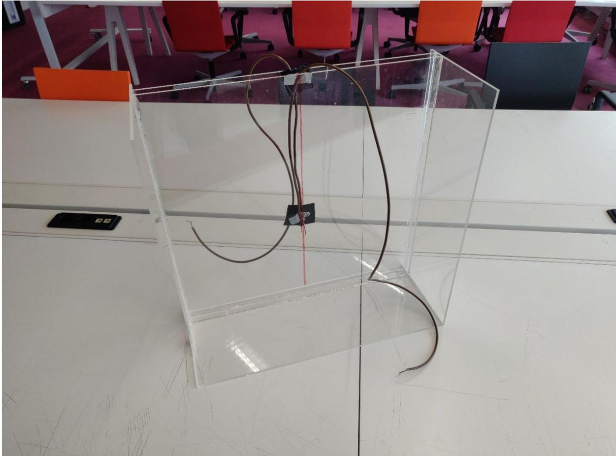
*Picture 4. PMMA box with thermocouples*
