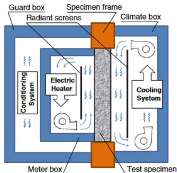
Figure 8. setup for dynamic hot-box testing. (Kośny, 2015)
