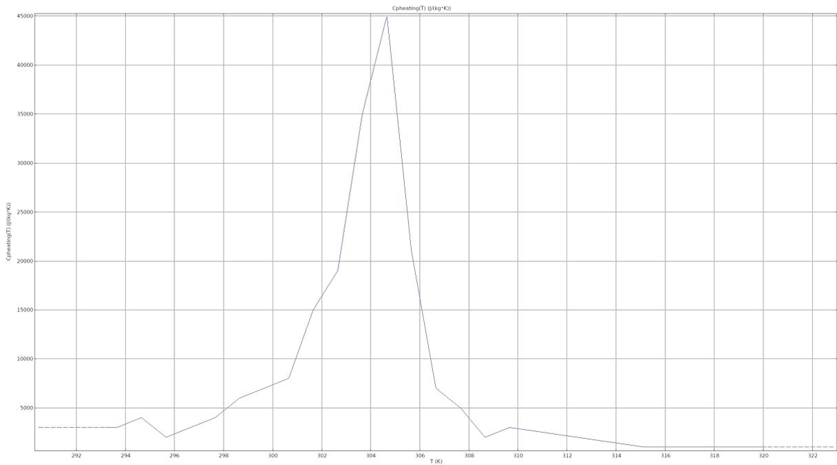
Figure 16: Temperature dependence of heat capacities  $C_{p,heating}$  for C28
