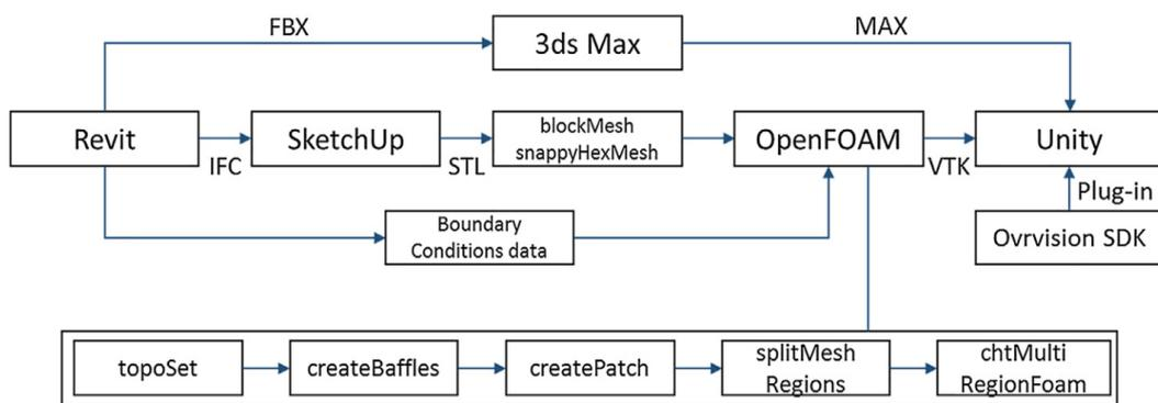
Figure 12. data flow for AR.(Fukuda et al., 2019)
