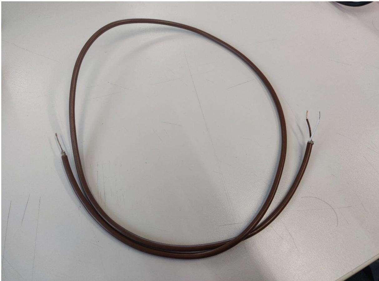
*Picture 3. Thermocouple type T*
