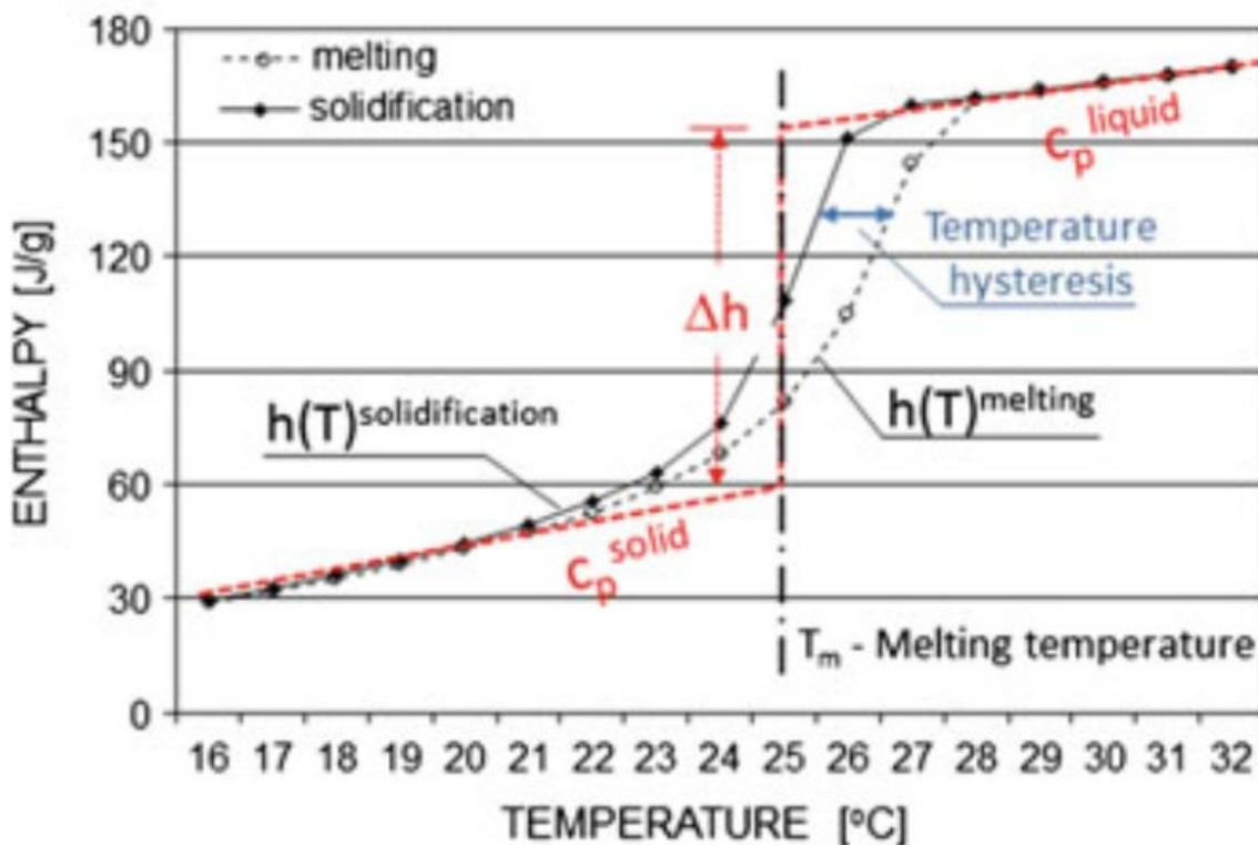
Figure 1. Enthalpy and temperature graph of a PCM (Kośny, 2015)
