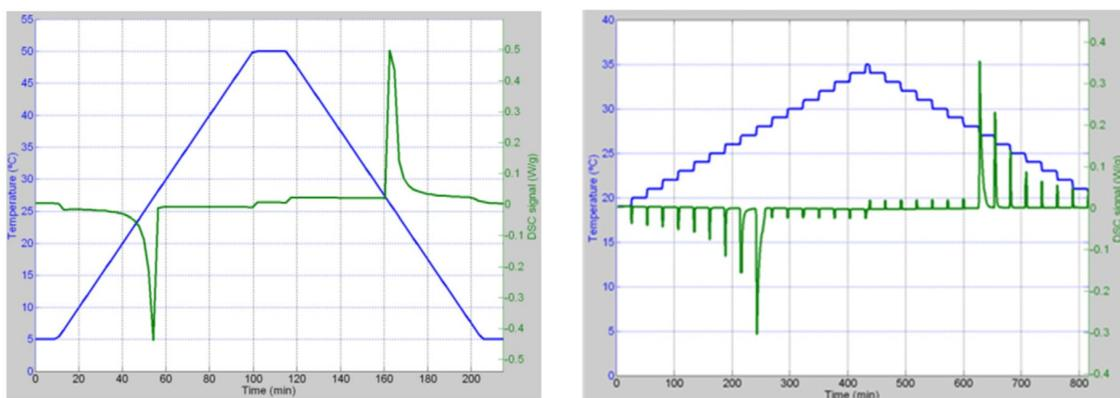
Figure 5. Dynamic(r) and step(l) DSC method. (Barreneche et al., 2013)
