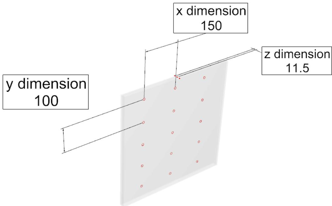
Figure 25. Dimensions of the thermocouples on the PCM container
