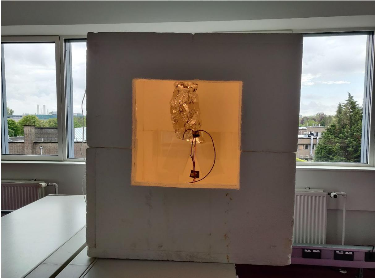
*Picture 5. Polystyrene box with setup*
